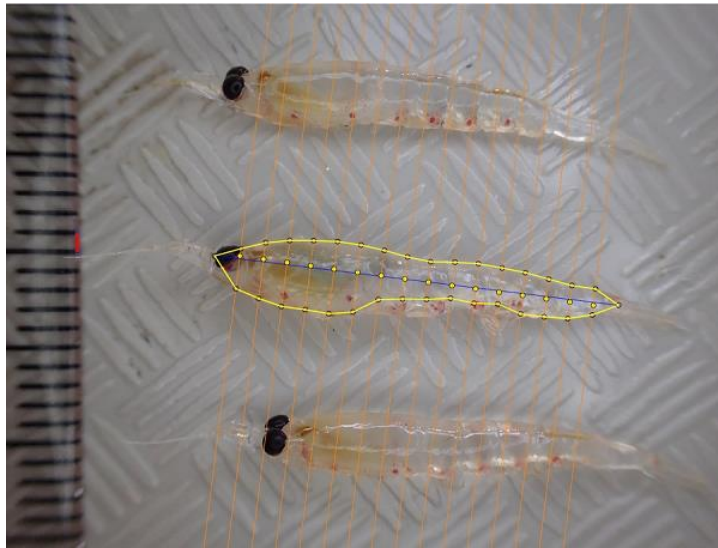
Figure 2. Animal shapes were measured from individual krill at 16 equidistant points along the animal's body. The red line represents a 1 mm calibration line, the yellow dots and orange lines represent the two-dimensional equidistant points used to approximate the discretized cylinders that parameterize TS models, and the yellow line represents the overall lateral two-dimensional shape of the animal.
