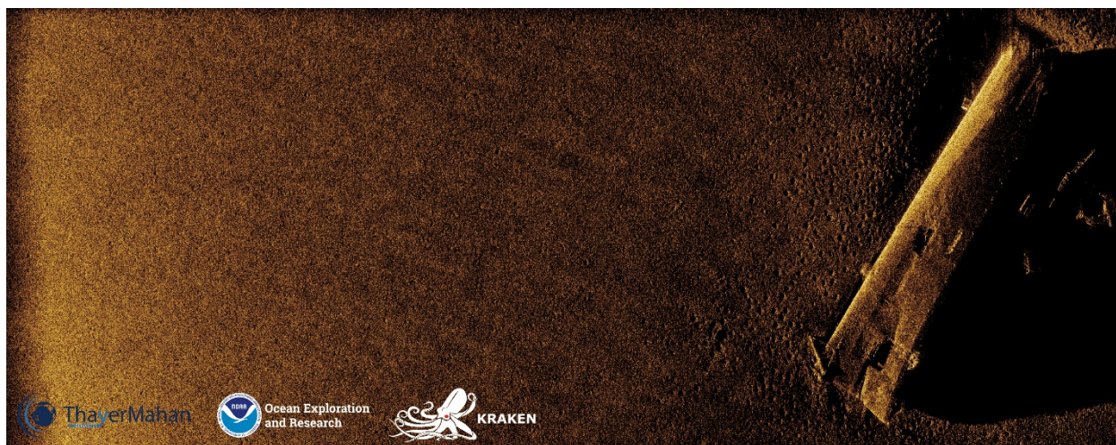
Figure 32. SAS image of the bow section of the USS Murphy that sank after the collision, lying on its port side. Note the biological burrows around the hull. Figure courtesy of ThayerMahan, Kraken, and OER.
