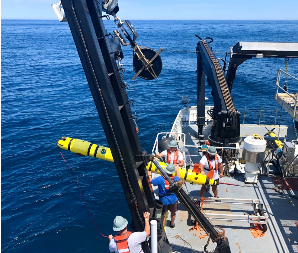
Figure 3. The REMUS 600 AUV was launched from the CTD deck using the J-frame and CTD winch. Image courtesy of Charles Wilkins.
