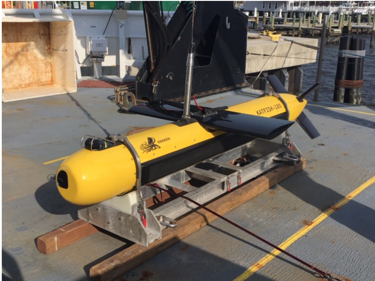
Figure 1. Towed KATFISH in cradle on the fantail. Image courtesy of B. Eakins, University of Colorado Boulder and NCEI.
