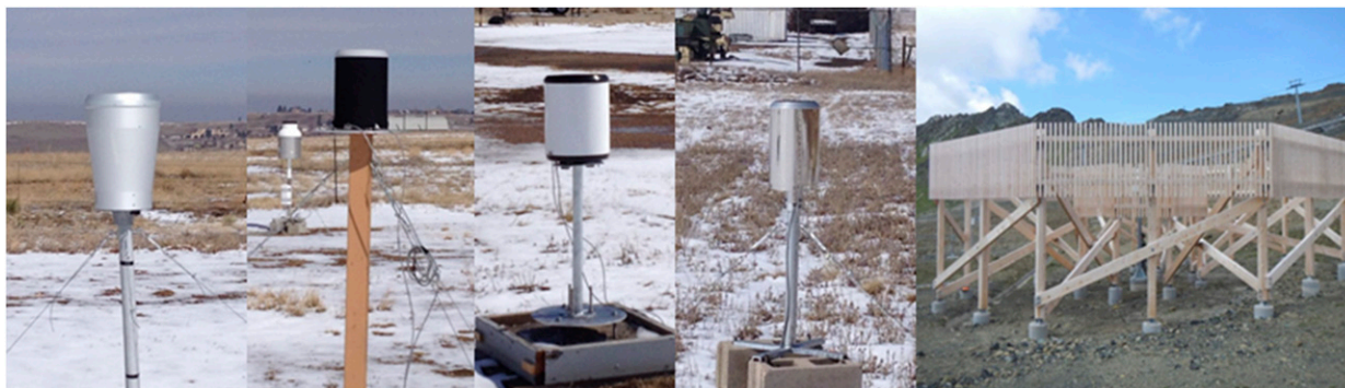
FIG. 2. Examples of the CAE, HSA, MR3H, Thies, and DFAR precipitation gauges (from left to right).
