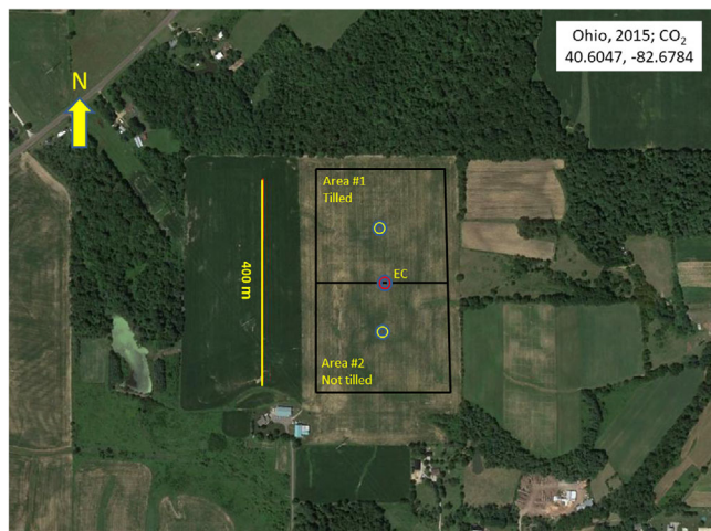
FIGURE 2 The surface layout of the test areas of the Ohio (2015) field study. White circles indicate the locations of Bowen ratio energy balance (BREB) measurement systems. The red circle shows where eddy-covariance measurements were made. The image is derived from Google Earth
