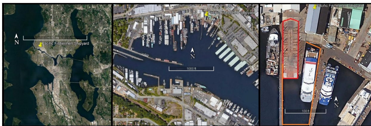
Figure 1. The Pacific Fishermen Shipyard dredging project site in the Lake Washington Ship Canal, Seattle Washington. The right image shows the dredging area outlined in red, and the full-depth sediment curtain location shown in orange.
