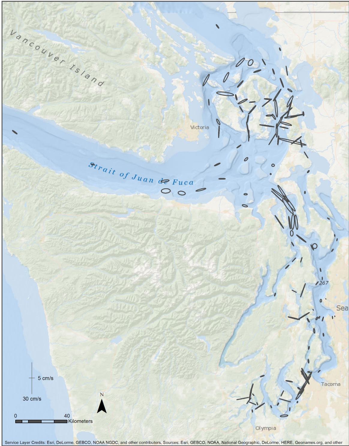
Figure 7-3. S_2 tidal ellipses for the entire study region. Note that these are on a different scale than M_2 in order to see the ellipses. These data are at \frac{1}{4} the scale of the M_2 data.
