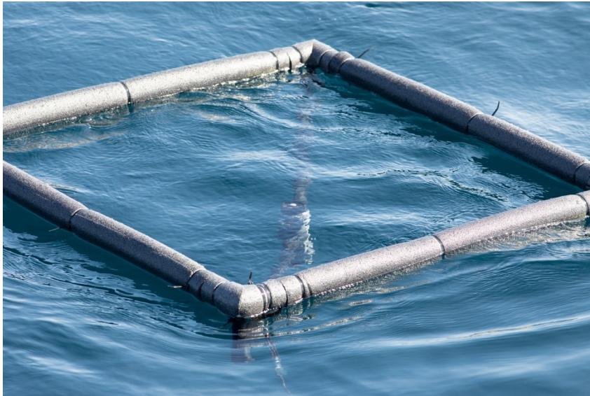
Figure 34. The RAMSES was held in the center of a floating frame with the height adjusted to keep the sensor head as close to the air-sea interface without breaking the surface.
