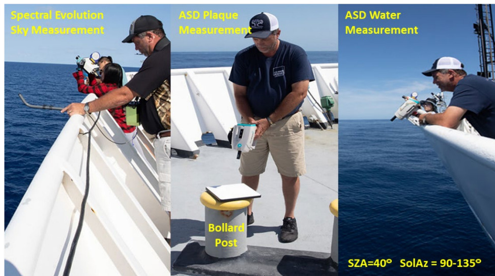
Figure 19. NRL group collection sequence (sky, plaque and water) during above water spectroradiometer (ASD and Spectral Evolution) data collection activities.
