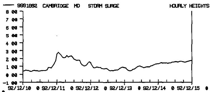
FIGURE 6. STORM SURGE - DECEMBER 1992 NORTHEASTER CHESAPEAKE BAY
