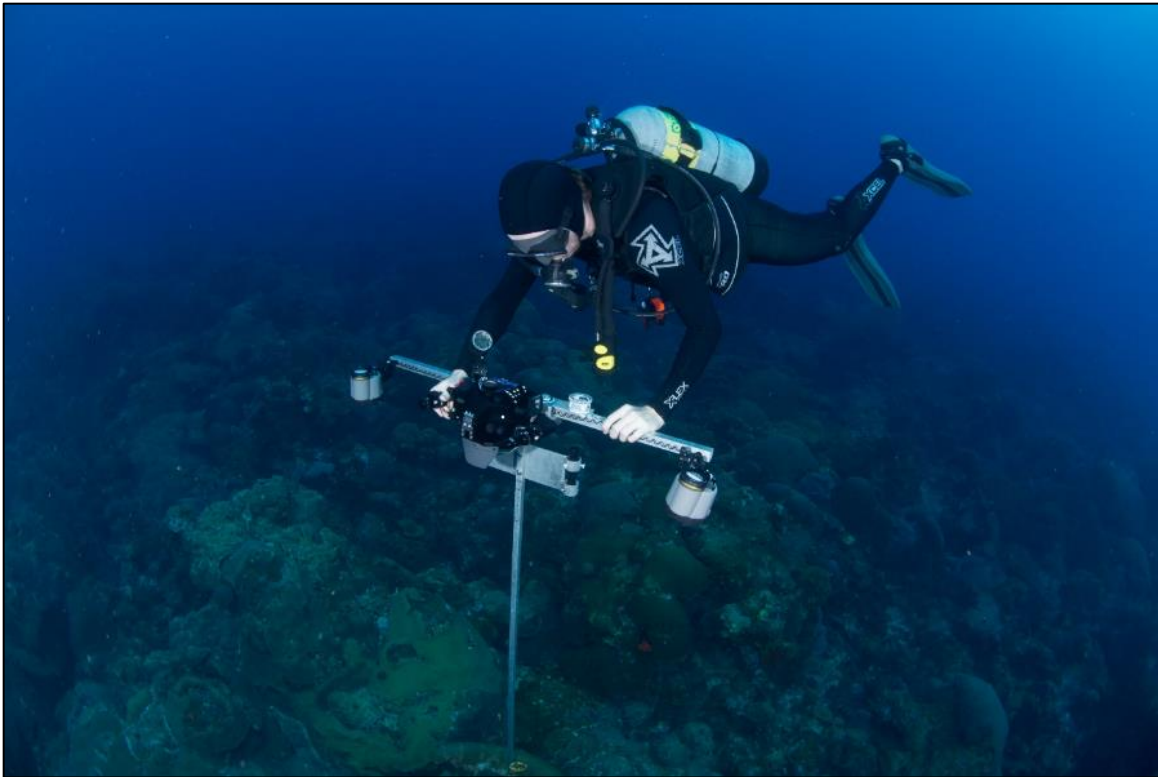
Figure 2.2. NOAA diver photographs a repetitive photostation with camera and strobes mounted to an aluminum t-frame. Photo: G.P. Schmahl/NOAA
