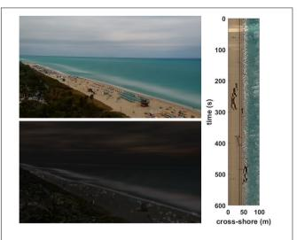
FIGURE 2 | An example time-exposure (top), time-variance (bottom) and time-stack (right) imagery from the Miami, FL webcarn at 1200 UTC on March 10, 2018. Note the white pixels varying along the beach that indicate where waves are breaking in the time-exposure image.
