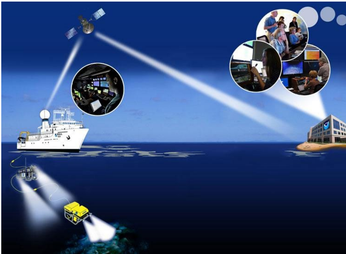
Figure 5. A telepresence-enabled platform: satellite technology enables data and video to be transmitted in real time, from NOAA Ship Okeanos Explorer and ROVs working at depth, to a shore-based hub where the video is transmitted in HD out on Internet2 to a variety of receiving stations on shore, including a number of Exploration Command Centers (ECCs) located around the country. A lower-resolution and higher-latency version is also available via standard Internet. Access to the video and a suite of Internet-based collaboration and communication tools allows scientists located on shore to join the operation in real time. Image courtesy of OER.
