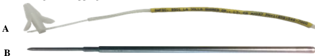
Figure 2. Conventional double-barbed plastic anchor BFIM- 96 Large Billfish Tag (A) printed with SWFSC contact information for recapture reporting, and accompanying BFIM-96 steel applicator tip (B). Tag and applicator tip shown are to scale.
