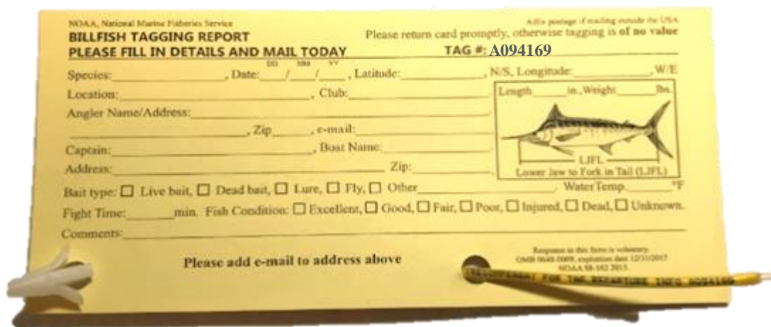
Figure 4. A tag-card unit for the conventional plastic anchor billfish tag, numbered A094169, and the accompanying labeled tag report card. Tag bundle is not to scale.
