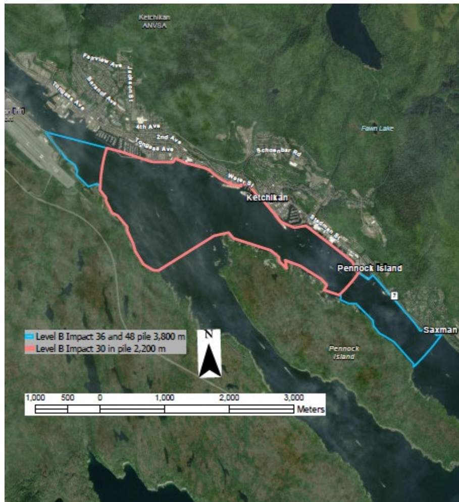
Figure 13. Level B monitoring zones for all impact pile driving of 30-in piles (pink, 2,200 m) and 36- and 48-inch piles (blue, 3,800 m) at COK Berth III (PND Engineers 2020b).
