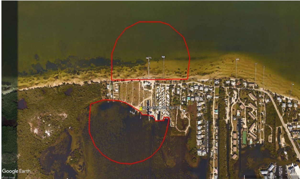
Figure 3. The Bocilla Island Seaport, surrounding area, and a 705-ft radius (in red) denoting the extent of the action area based on behavioral noise effects to ESA-listed fishes (©2020 Google Earth)
