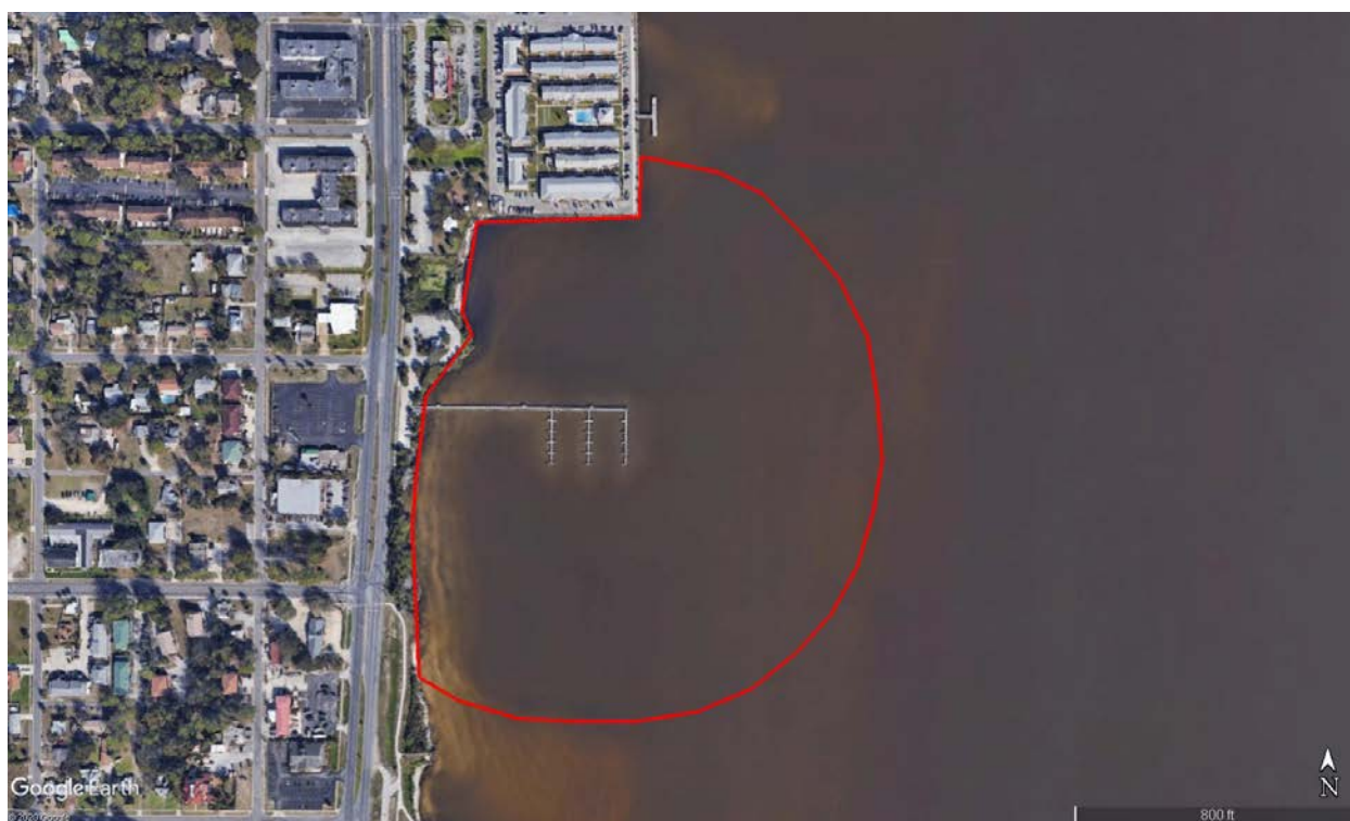
Figure 1. The Rotary Riverfront Park Fishing Pier, surrounding area, and a 705-ft radius (in red) denoting the extent of the action area based on behavioral noise effects to ESA-listed fishes (©2020 Google Earth)
