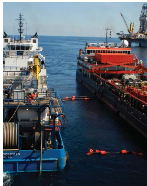
GULF OF MEXICO – The crew of Blue Dolphin and the HOS Centerline pump mud through lines to the Q4000 and down to the temporary cap and into the well for a static kill, as the DD II crew continues to drill a relief well in the background. Photo courtesy of the U.S. Coast Guard
