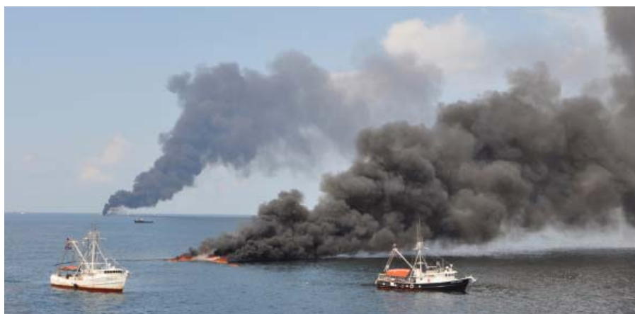
GULF OF MEXICO – Vessels of Opportunity pull oil into a fire boom in a controlled burn with a second controlled burn visible in the distance. Photo courtesy of U.S. Coast Guard
