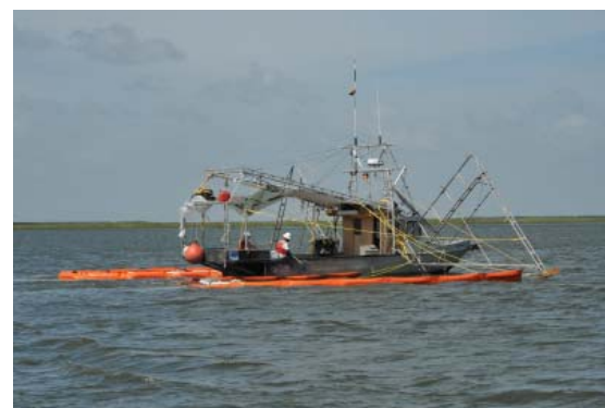
RIGOLETS, La. - A fishing vessel equipped with skimmers makes its way up and down the Rigolets as a precautionary measure to capture any stray tar balls. Photo courtesy of U.S. Coast Guard
