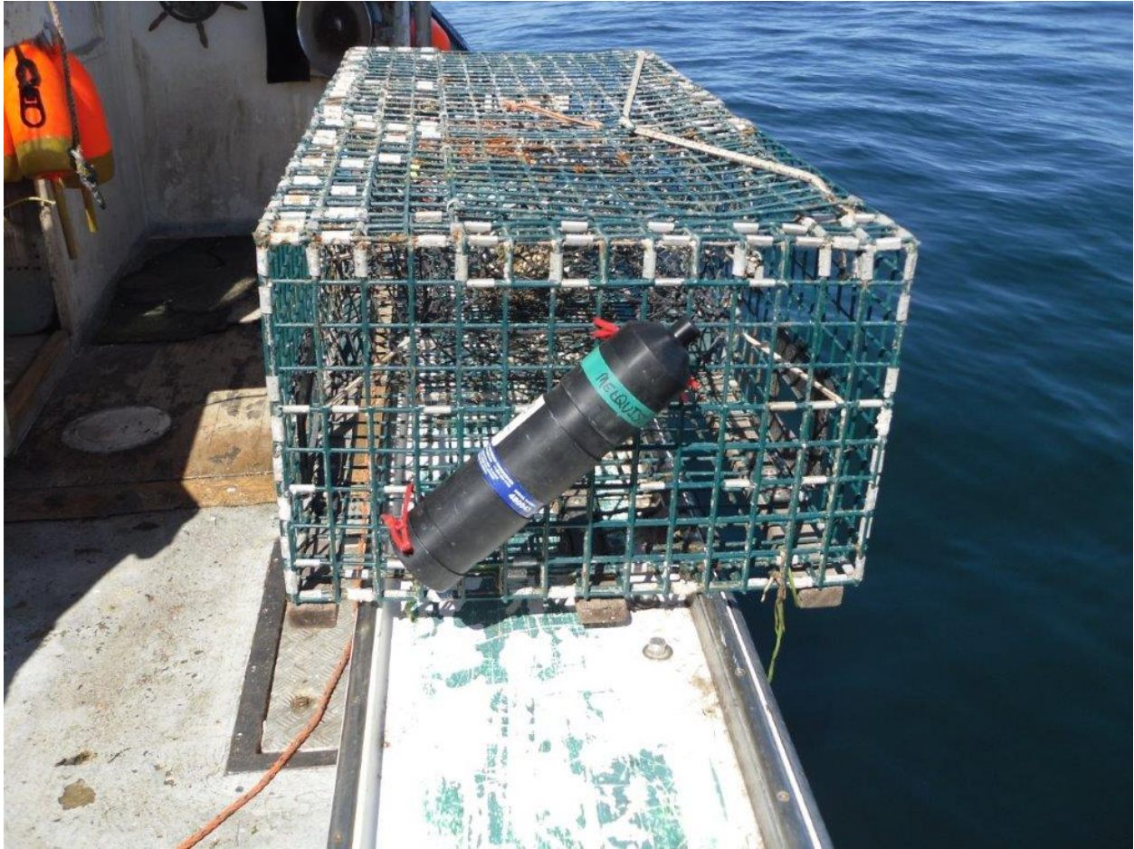
Figure 3. An acoustic receiver (VR2W) attached to a lobster trap – ready for deployment. Photo Credit – John Melquist Sr.
