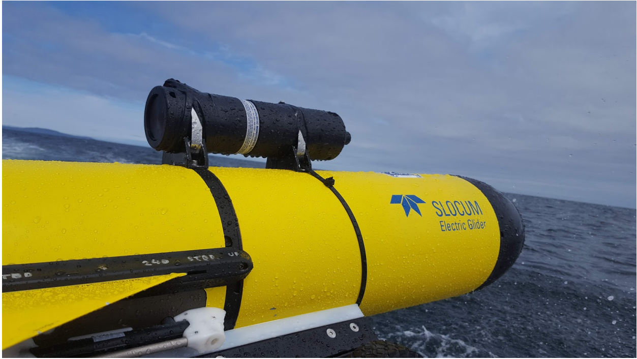
Figure 5. A G2 Teledyne Webb Slocum glider retrofitted with an InnovaSea VR2W receiver before deployment off of Northeast Harbor, ME.
