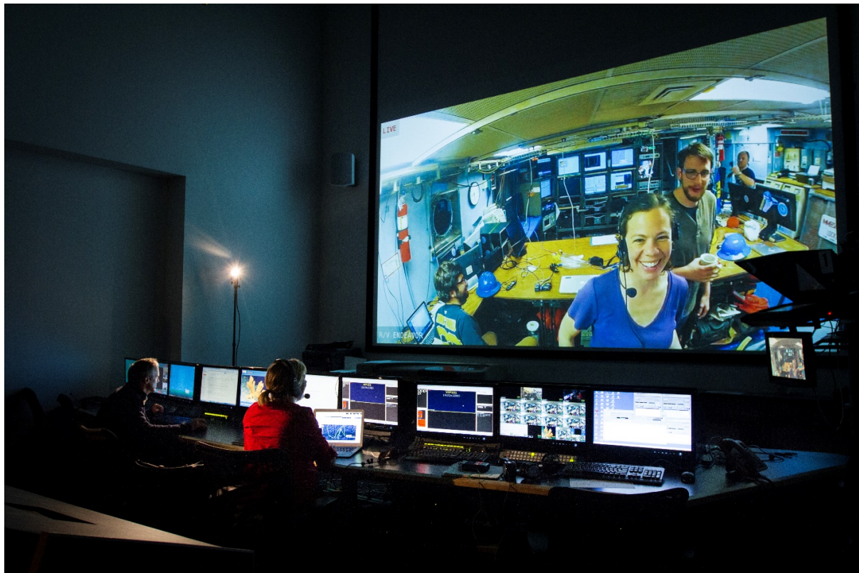
Figure 3. Mission Control at the URI Inner Space Center: A large projection screen can display multiple live feeds of video, data, and supporting information. ISC and mission personnel work at science stations, where they have access to multiple computers, video recording and playback devices, and intercom systems for communicating with telepresence-enabled ships at sea, and other participating ECCs. Currently, the ISC can host up to 15 on-site participants. Photo courtesy of Alex DeCiccio, Inner Space Center.
