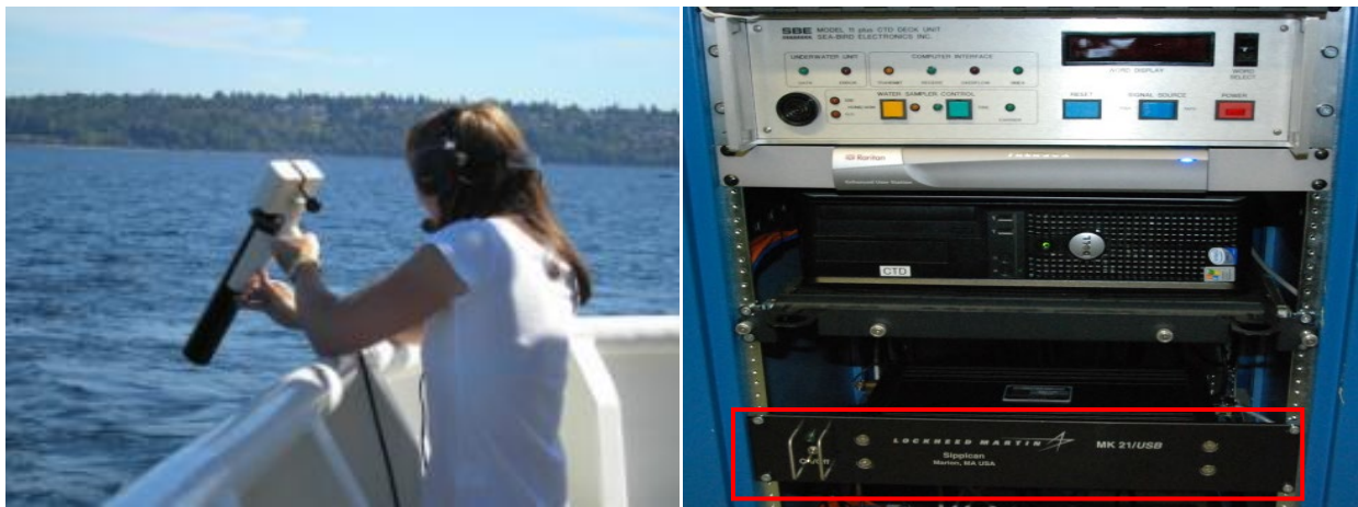
Figure 2. Sippican XBT launch from the aft deck (left). Deck unit for Sippican XBT (right).
