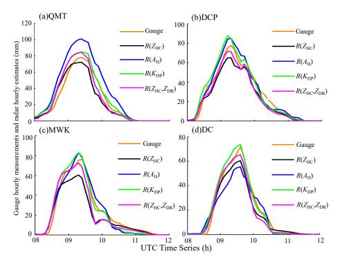
**Figure 9.** Gauge hourly rainfall measurements and corresponding radar estimates using  $R(Z_{HC})$ ,  $R(Z_{HC}, Z_{DR})$ ,  $R(K_{DP})$ , and  $R(A_H)$  at each gauge station during from 08:00–12:00 UTC, 23 June 2015: (a) station QMT; (b) station DCP; (c) station MWK; and (d) station DC.
