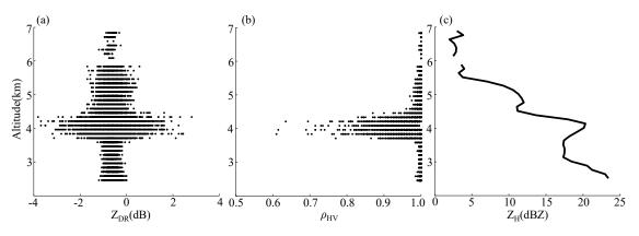
**Figure 2.** Vertical distribution of radar measurements from a "birdbath" scan at 1835 UTC, 24 April 2015: (a)  $Z_{DR}$ ; (b)  $\rho_{HV}$ ; and (c)  $Z_{H}$ .
