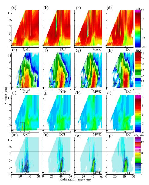
**Figure 5.** (**a**–**d**) are the vertical cross-section (VCS) of *V*r along radial directions from the DMM radar to QMT, DCP, MWK, and DC at 0829 UTC, 23 June 2015. (**e**–**h**), (**i**–**l**), and (**m**–**p**) are the VCS of  $Z_H$ ,  $Z_{DR}$ ,  $K_{DP}$ , respectively, at the same time. DMM radar is marked with "+" at the y-axis, and the distances of four gauge stations are marked with "+" along the x-axis. The rectangle in (i) refers to the  $Z_{DR}$  column near the convergence line.
