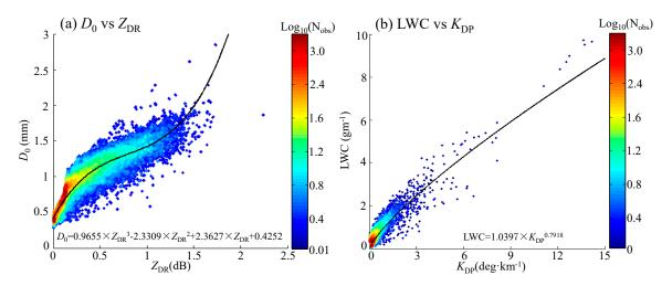
**Figure 11.** Scatter density plots of simulated variables based on DSD data: (a)  $D_0$  vs.  $Z_{DR}$  and (b) LWC vs.  $K_{DP}$ .
