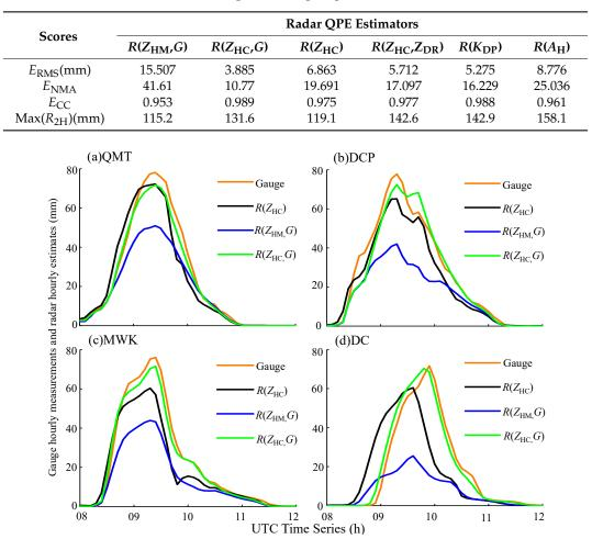
Table 1. Information of six radar quantitative precipitation estimation (QPE) estimators.
