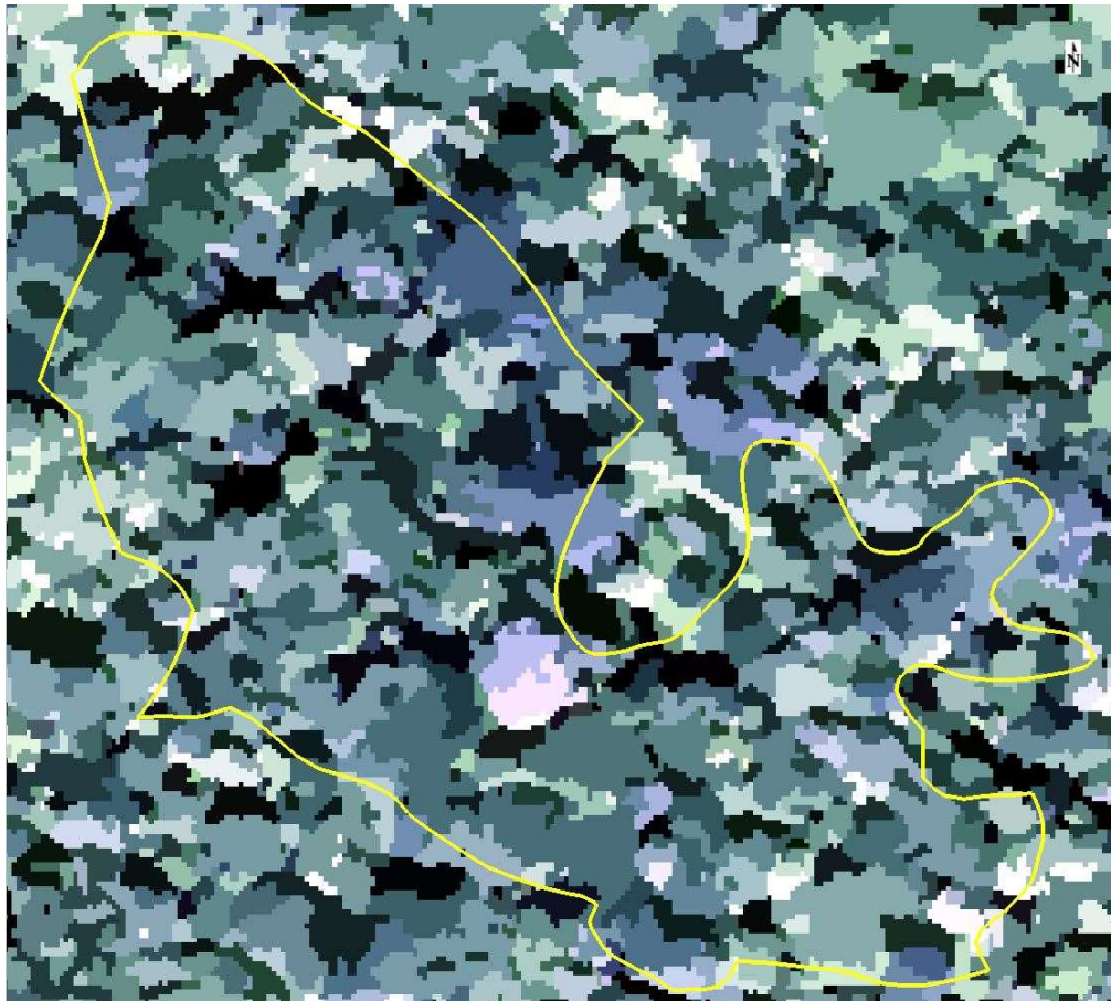
Figure 7. The result of the ENVI segmentation process for the Arboretum based on a setting of 11 for scale and 86 for merge in the segmentation settings. Each defined colored segmented feature represents an object in the image with like qualities and reflective properties. The values of the two SVIs defined the segments (Table 4), maximizing the differentiation in the imagery between features.
