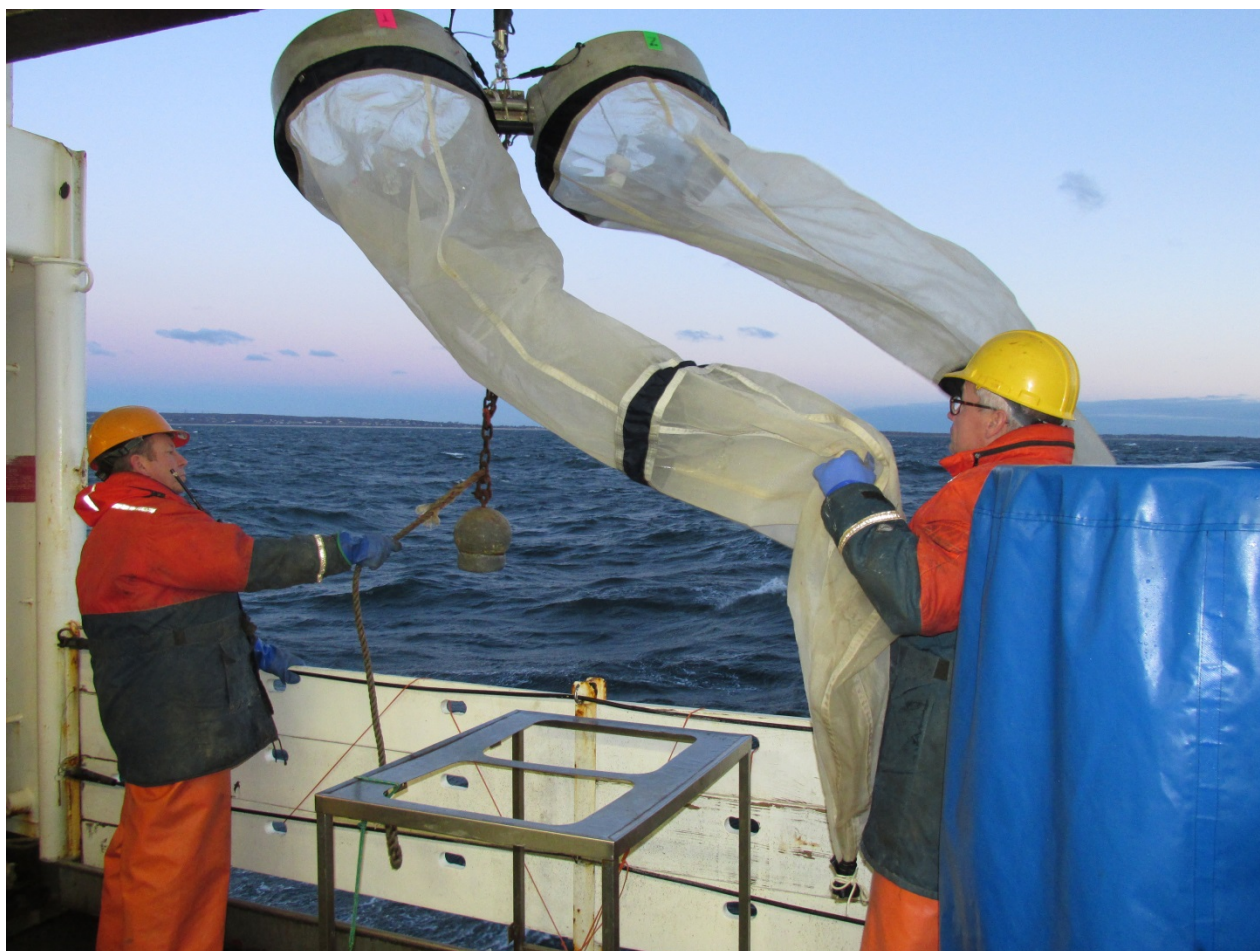
Figure 2. Bongo net array, showing 61 cm bongo nets being deployed from the port side of the FSV Henry Bigelow .
