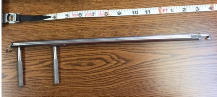
Figure 1.1.3. Example of new sea turtle dehooker to release incidentally hooked sea turtles. Photo credit: NMFS-SEFSC.
