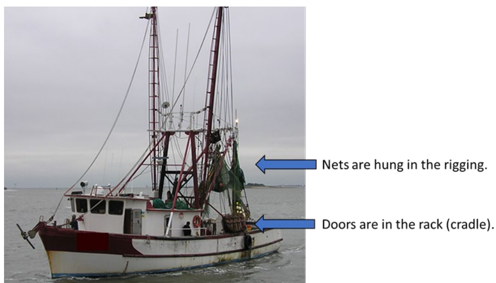
Figure 1.1.1.2. Picture of shrimp vessel with trawl doors in the rack (cradle) and nets tied up and hung in the rigging. Try net not pictured here. Represents the stowage requirement for proposed Preferred Option 2 . Credit: South Atlantic Fishery Management Council.
