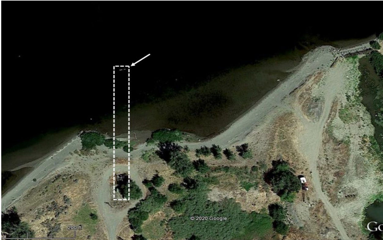
Figure 2. N&C Irrigation Intake Pipeline footprint at project site. The white dotted outline represents the footprint where the excavation and construction for the intake pipeline and screen replacement will occur.
