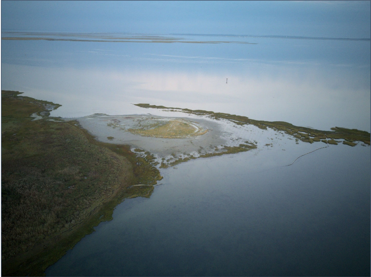
Figure 25. Sediment placement area near the northern end of Mordecai Island. During higher tides, the boundary between the placement region and northern lobe of the island is flooded all the way across.
