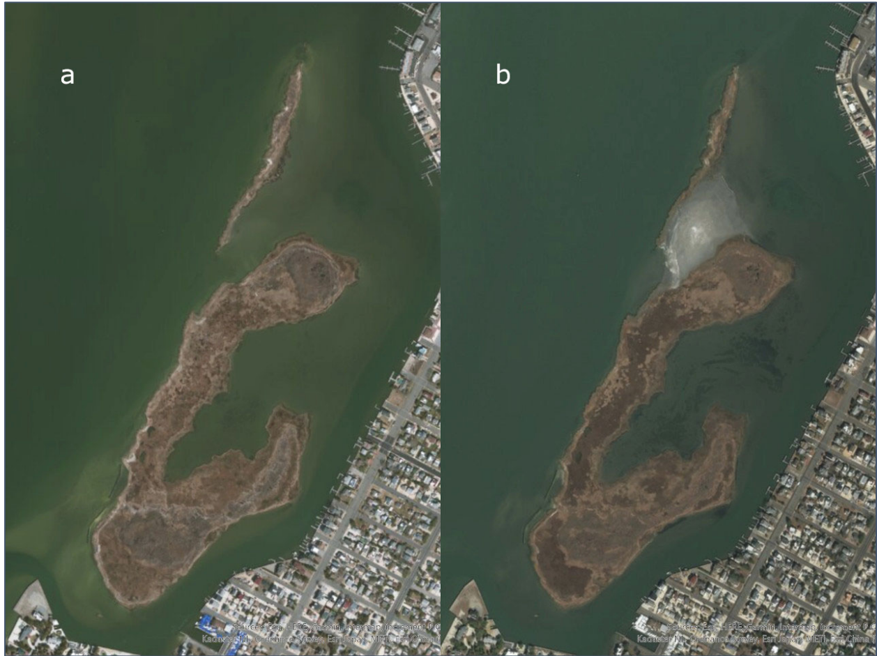
Figure 1. Aerial images depicting Mordecai Island before (a) and after (b) dredged sediment placement. Image source: ESRI World Imagery; 02-20-2014 and 01-08-2018.
