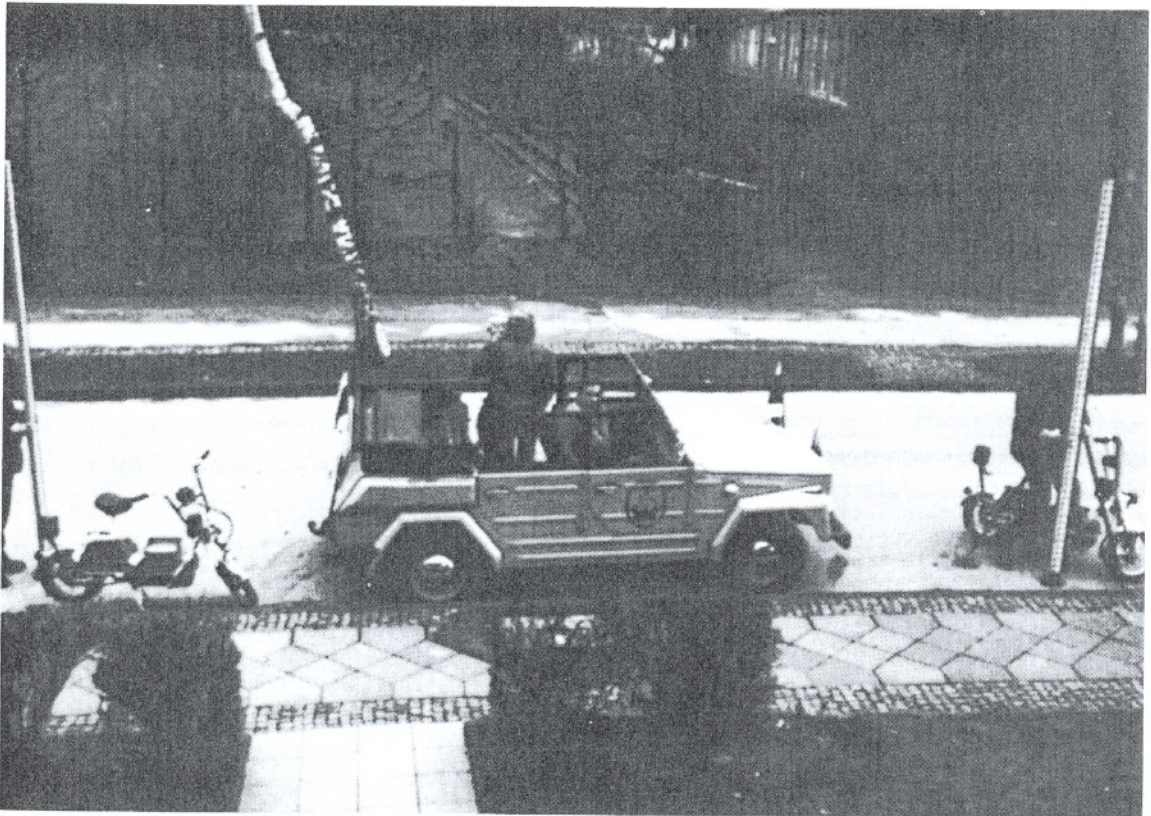
Figure 3.--Motorized leveling being performed by means of one compact car and two electric motorbikes. (Courtesy: Dr.-Ing. H. Wesemann, Federal Republic of Germany)
