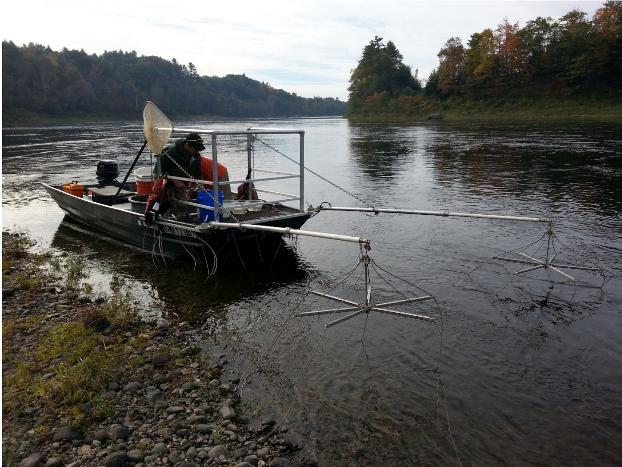
Figure 1. The electrofishing boat used by MBI to sample fish assemblages in the Lower Kennebec River showing the electrofishing booms with the umbrella anode dropper and bow cathode curtain arrays.
