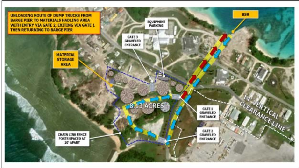
Figure 4. Barge unloading route
