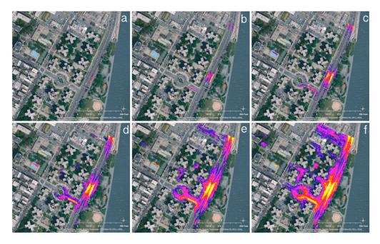
**Figure 6.** Expected flooded area (EFA) for base level (Lowli) and subsequent  $\Delta L = 15.25$ cm increments Basin53—(a) Lowest topographic level—Lowl1 = 1.62 m, EFA = 500 m<sup>2</sup>; (b) Lowl2 = 1.77 m, EFA = 3745 m<sup>2</sup>; (c) Lowl3 = 1.92 m, EFA = 12,228 m<sup>2</sup>; (d) Lowl4 = 2.08 m, EFA = 32,834 m<sup>2</sup>; (e) Lowl5 = 2.23 m, EFA = 63,649 m<sup>2</sup>; (f) Lowl6 = 2.39 m, EFA = 102,251 m<sup>2</sup>.
