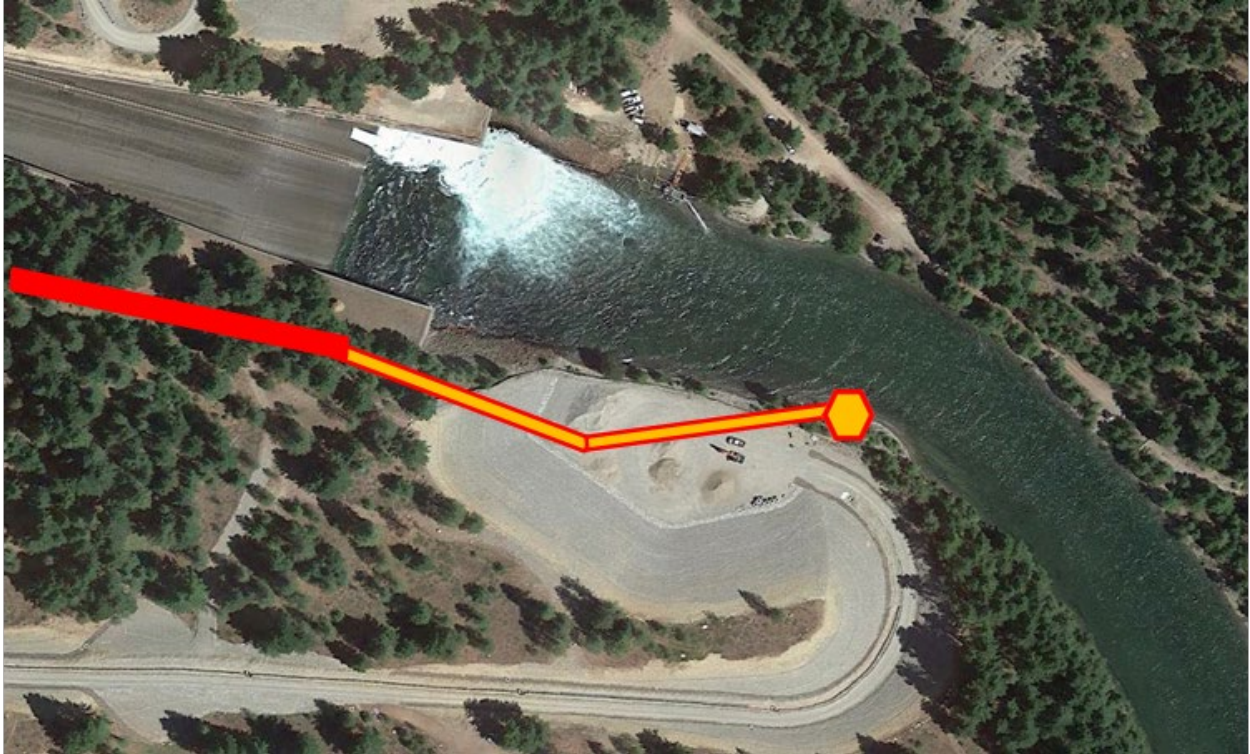
Figure 2. The Helix Bypass Pipe (yellow) will be connected to the Juvenile Passage Tunnel (red) and discharge into the river at the dissipation pool (yellow hexagon) (Reclamation 2020, their Figure 11).
