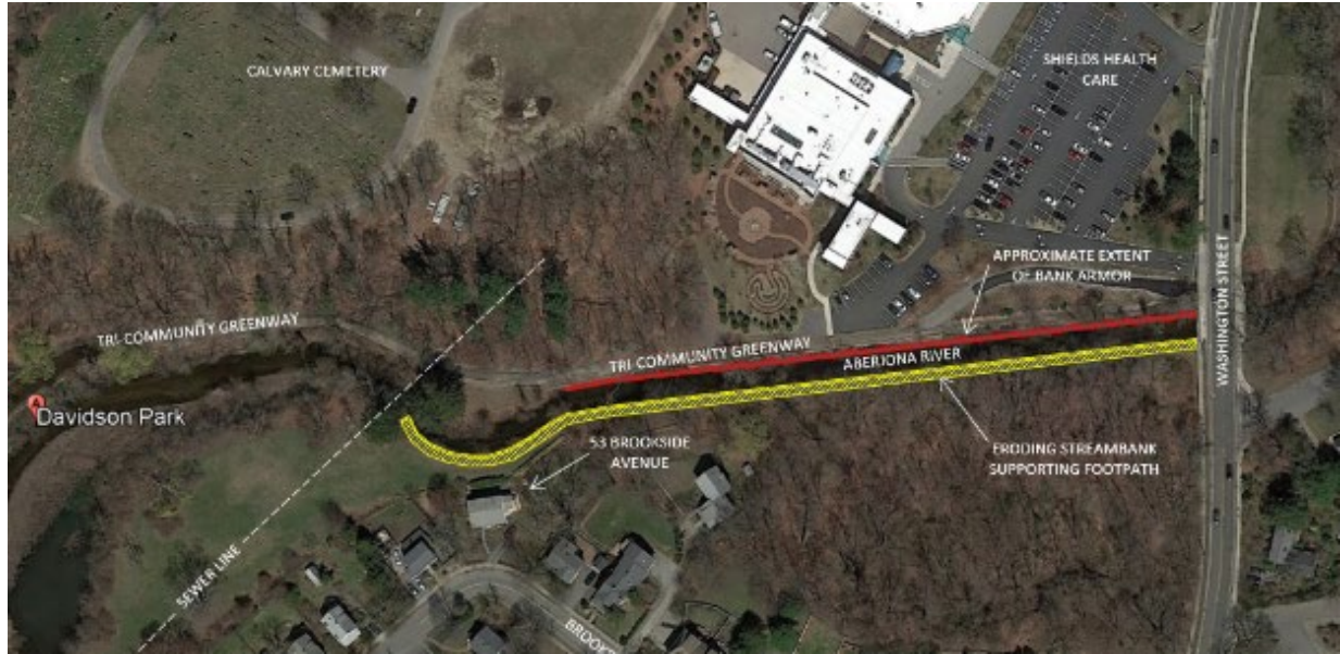
Figure 9. Map of the Northeast End of Davidson Park, Showing the Greenway and the Area of Erosion along the Opposite Bank of the Aberjona River
