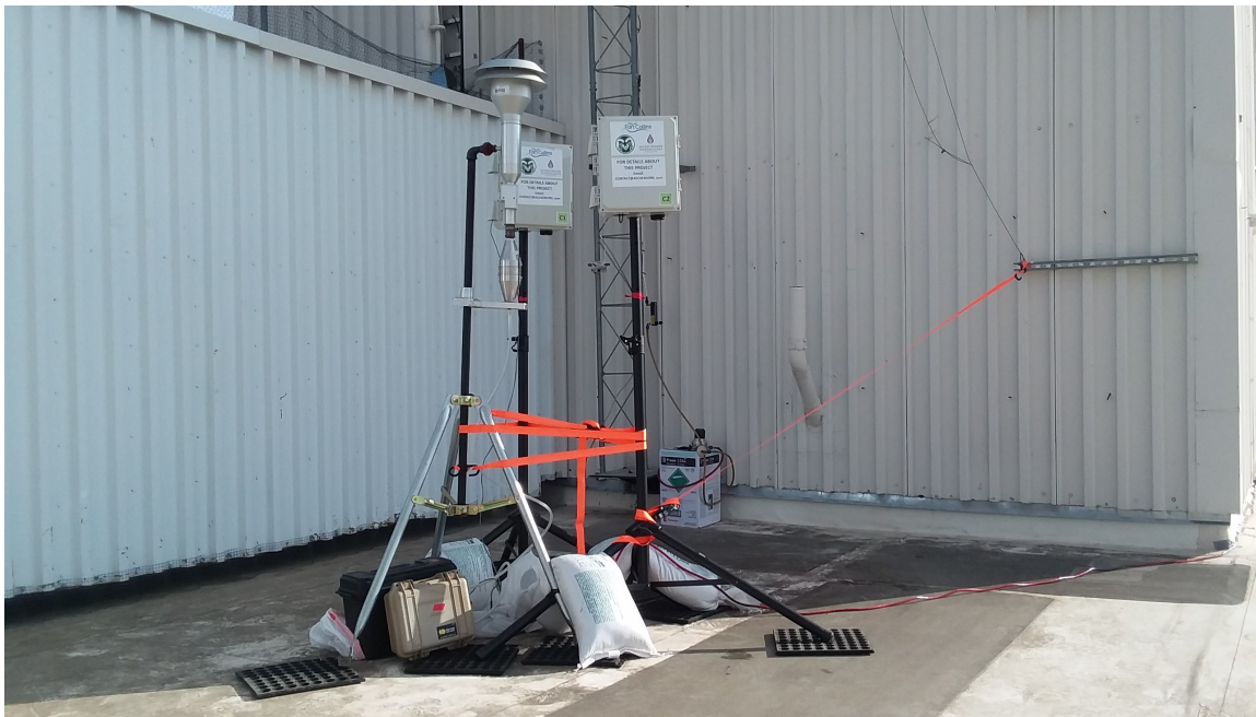
Figure S3. Two ASPEN boxes and one 16.7 \text{ L min}^{-1} filter sampler co-located at site C.
