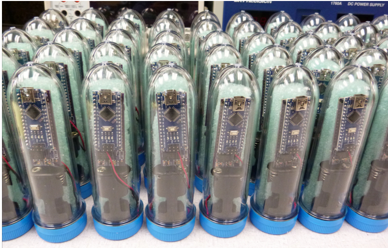
Figure 1. Assembled thermistors arrayed in the lab, ready for deployment.
