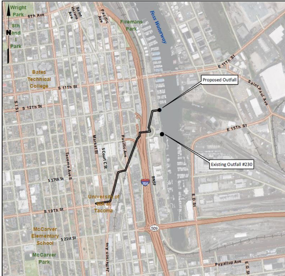
Figure 1. Google satellite photographs of the Foss waterway with location of existing and proposed new outfalls identified. Pathway of the new conveyance system is denoted as a black line.
