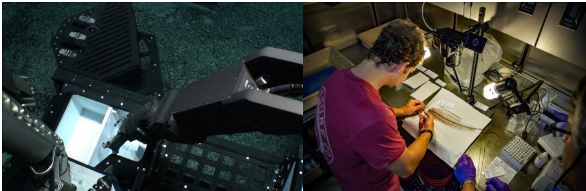
Figure 3. Left: Manipulator arm and sampling box of the ROV Deep Discoverer , which were used to collect samples during ROV seafloor surveys. Right: Processing of collected specimens in the wet lab of NOAA Ship Okeanos Explorer .
