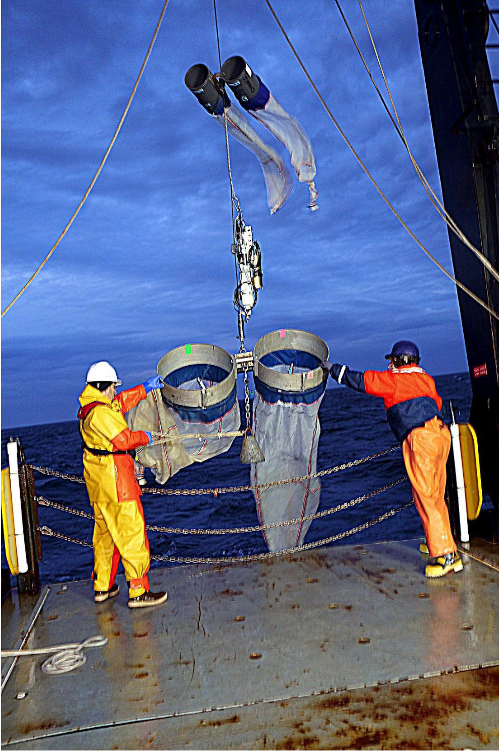
Figure 2. 61 and 20 cm bongo net array being deployed from the stern of the R/V Sharp.
