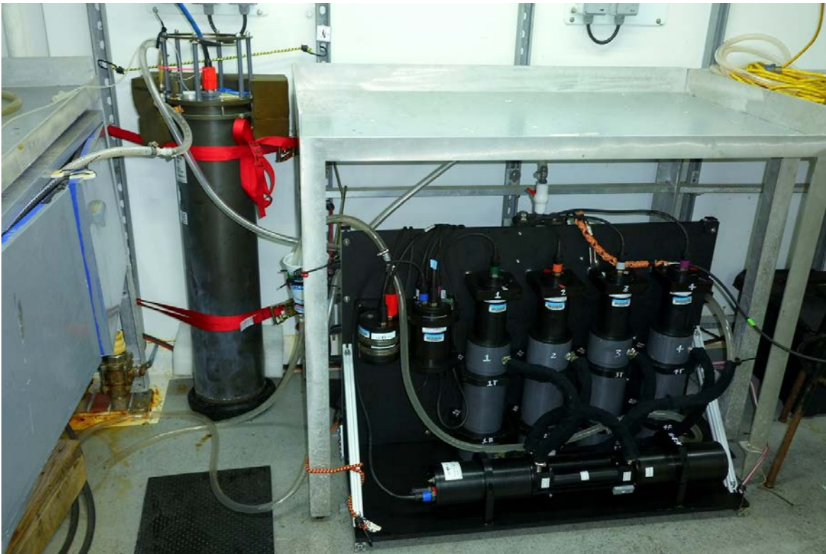
Figure 5. ImagingFlowCytoBot (tall gray cylinder) and URI seawater optical sensor array in the Sharp wetlab.
