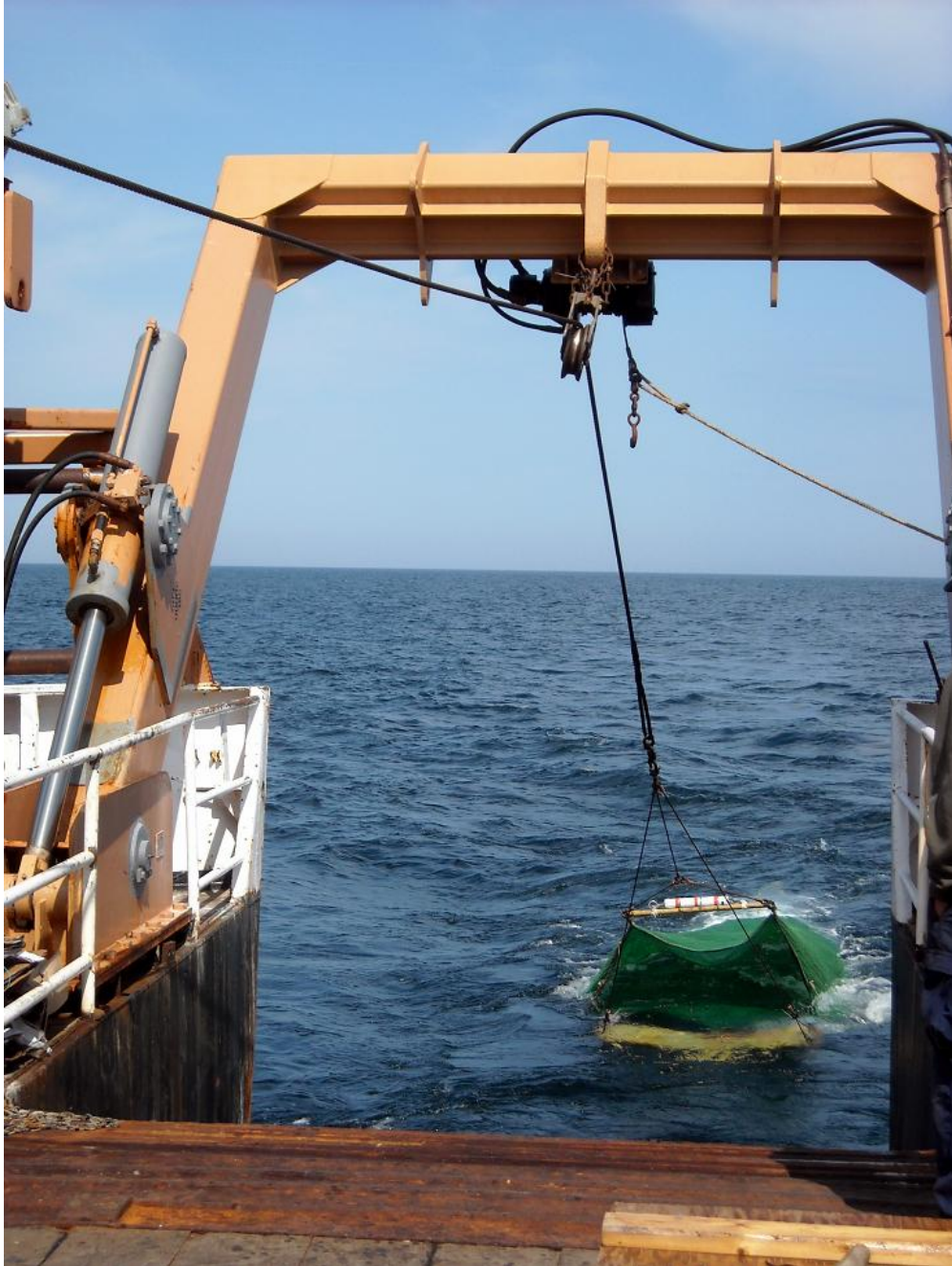
Figure 3. Isaacs Kidd Midwater Trawl being retrieved up the stern ramp aboard the Delaware II. Note CTD 19 unit on spreader bar.
