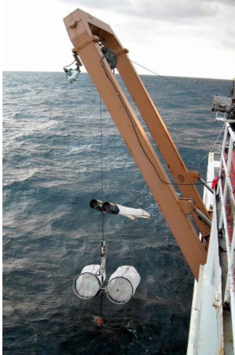
Figure 2. Bongo net array being retrieved aboard from the starboard A-frame of the Delaware II, showing 61 and 20 cm bongo nets, CTD unit and bell shaped depressor weight.
