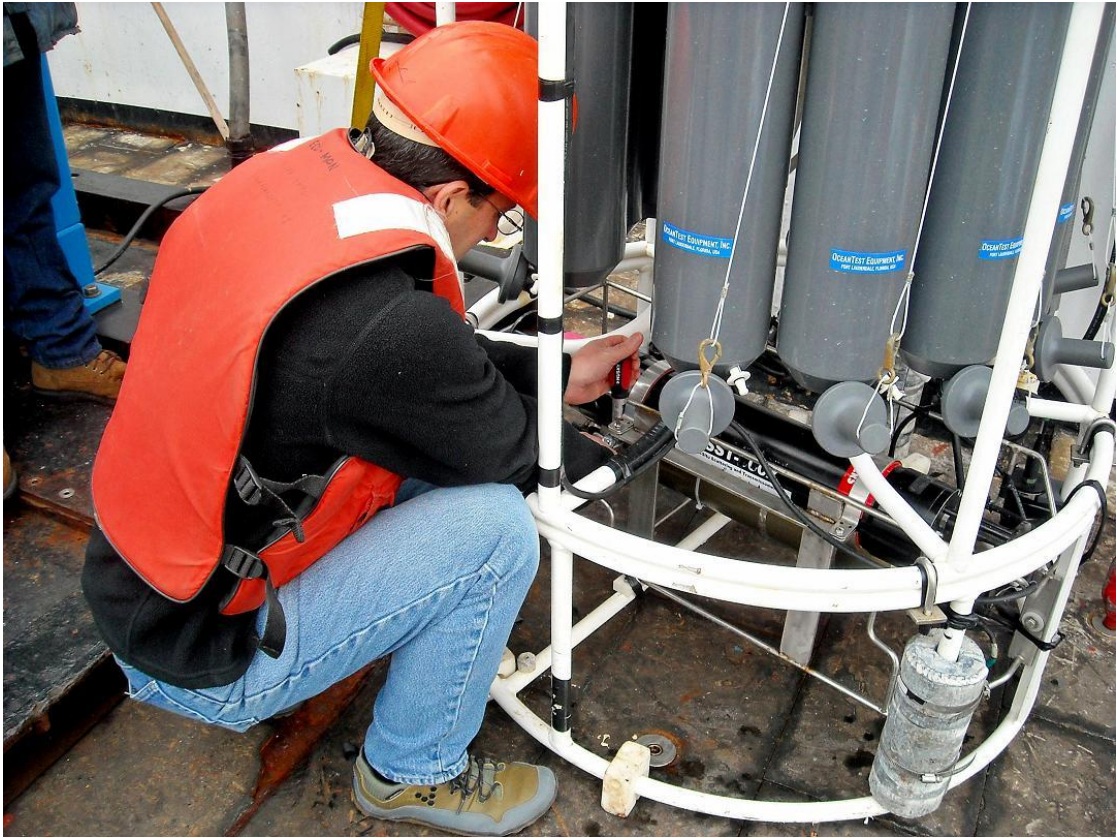
Figure 4. LISST unit (black cylinder) mounted underneath Niskin bottles on bottom of rosette.
