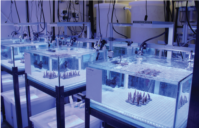
The Experimental Reef Laboratory, associated with NOAA's Atlantic Oceanographic and Meteorological Laboratory and the University of Miami, allows scientists to vary coral stress and measure molecular-level responses to identify resilient strains that may be used in restoration efforts.
