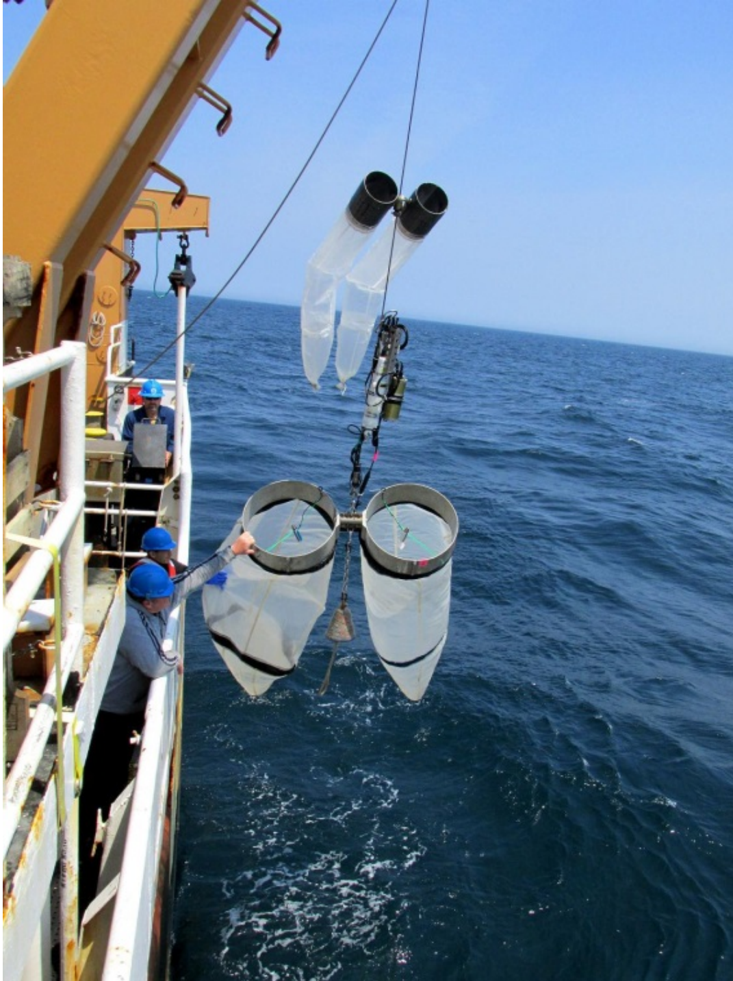
Figure 2. Bongo net array, showing 61 and 20 cm bongo nets being deployed from the port side of the FSV Gordon Gunter .
