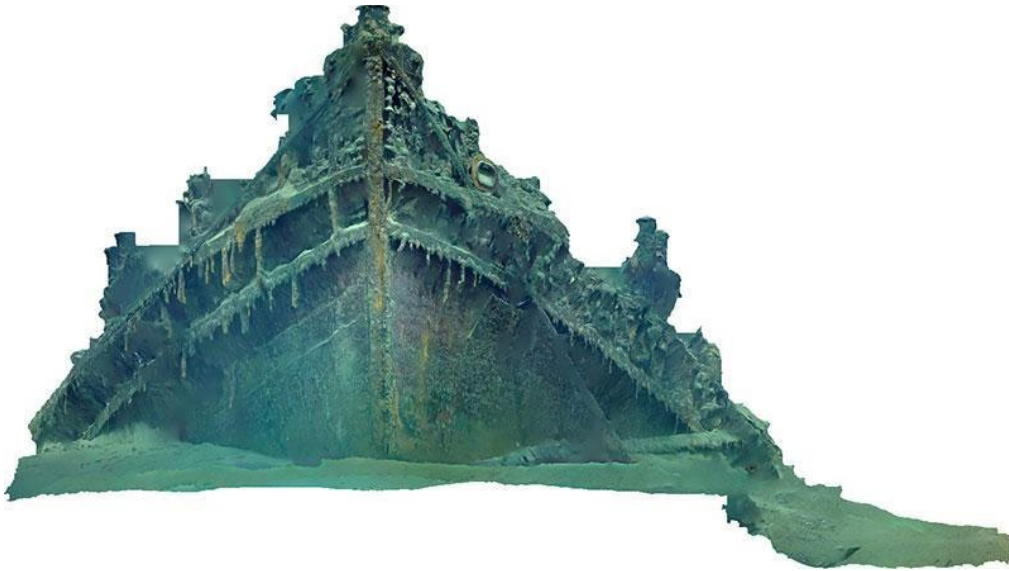
Figure 5. Orthophoto showing the bow of the tugboat New Hope , generated using imagery collected during Dive 01 of the expedition. This kind of orthomosaic is a series of individual photos which are matched using thousands of points to form a new 2D composite image consisting of all the smaller images, but with any distortion from perspective shift removed. Image courtesy of the NOAA Office of Ocean Exploration and Research, Gulf of Mexico 2018
