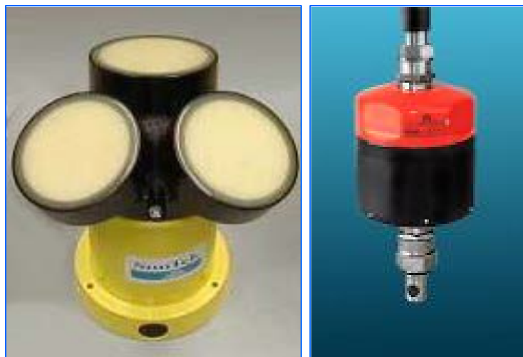
Figure 3-2. SonTek ADP (left); Aanderaa Doppler current sensors (right).
