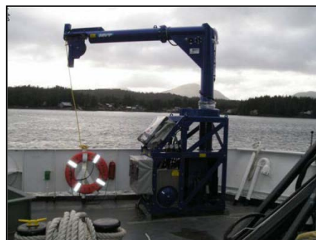
Figure 10. Moving vessel profiler mounted on fantail
