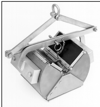
Figure 7. 6" x 6" Ponar Wildco grab sampler
