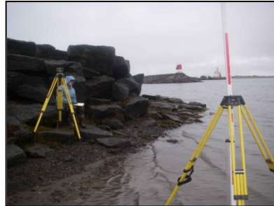
Figure 13. Leveling a tide gauge
