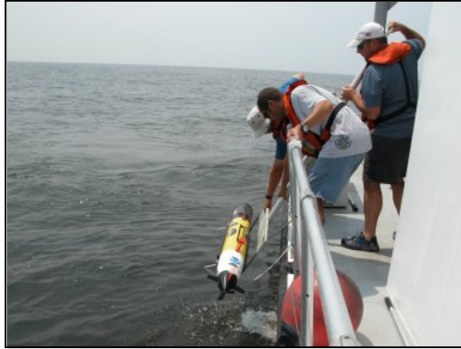
Figure 15. Hydrographers deploy an autonomous underwater vehicle
