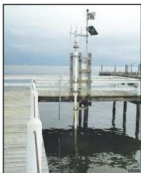
Figure 11. Pier-mounted acoustic sensor tide gauge
