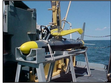
Figure 4. L-3 Klein 5000 side scan sonar
