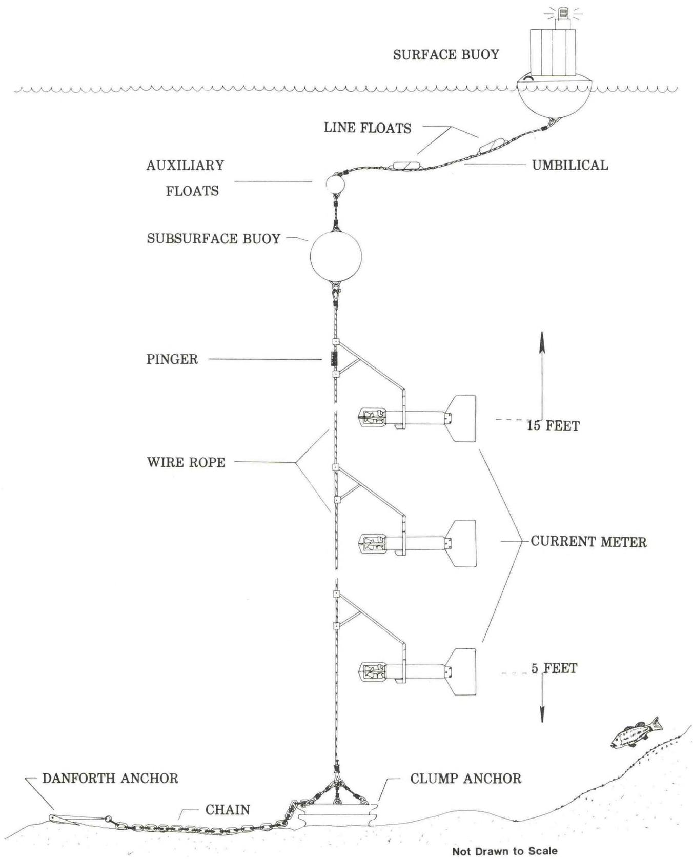
Figure 8.--Current Meter Taut-Wire Mooring System
