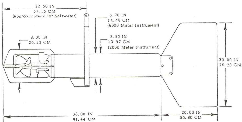
Figure 6.--Grundy 9021 G Current Meter Dimensions
