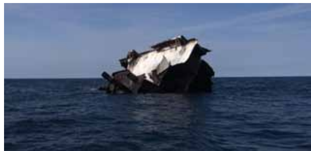
Figures 39 and 40. The shipwreck Nordmeer (1954-1966; 35-foot depth) rests on Thunder Bay Island Shoal, where ice and waves have battered the steel vessel for 44 years. The image at left was taken just after the vessel ran aground. By 2010, only a small portion of the vessel remained above the surface (right), but this too finally succumbed to natural processes, leaving the entire wreck today collapsed below the water's surface.
