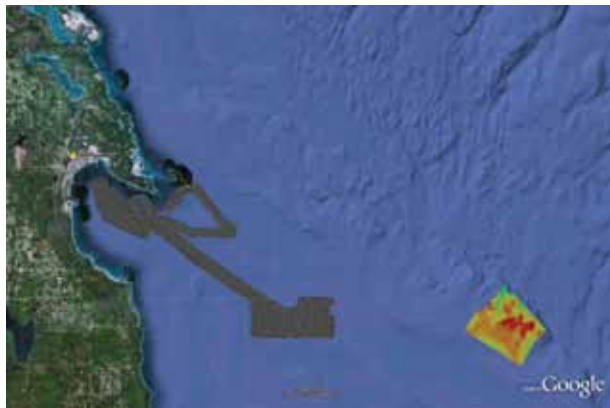
Figures 53 and 54. Two separate remote sensing efforts in 2010 resulted in the discovery of one new shipwreck and an enhanced understanding of a submerged land bridge that runs across Lake Huron. The darker area (left) represents sonar data acquired with a forward-looking sonar mounted on a REMUS 600 autonomous underwater vehicle (right). The 52-hour survey covered 104 square miles at an average rate of two square miles per hour. The colored area in the image on the left is multibeam data acquired using the sanctuary's R/V Storm. Logging 52 hours of survey time, the team mapped 46 square miles.
