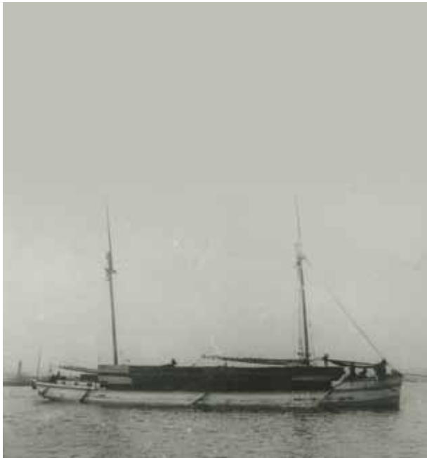
Figure 8. Originally built as a three-masted schooner, the 162-foot Harvey Bissell was later retrofitted to a two-masted “schooner barge,” a typical conversion for schooners whose owners sought to keep the aging vessels in use. Note the tow line at the bow extending out of the right frame of the photograph. Pictured here with an enormous deck load of lumber, the Bissell wreck sits in 15 feet of water just off the Alpena waterfront.
