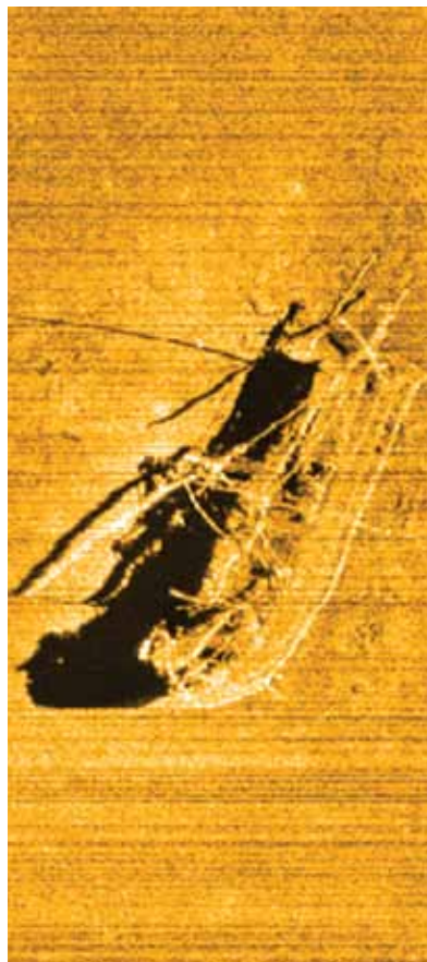
Figure 57, 58, and 59. Left: Site assessments are conducted using a variety of data, from sonar images to direct observation by divers. This side-scan sonar image of the schooner M. F. Merrick (discovered by the sanctuary in 2011) is a good example and offers much useful data. At 300 feet deep, the wreck's assessment relied chiefly on this image, which in turn informed follow-up ROV and SCUBA dives to the site.
