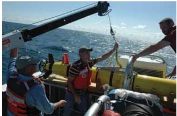
Figures 53 and 54. Two separate remote sensing efforts in 2010 resulted in the discovery of one new shipwreck and an enhanced understanding of a submerged land bridge that runs across Lake Huron. The darker area (left) represents sonar data acquired with a forward-looking sonar mounted on a REMUS 600 autonomous underwater vehicle (right). The 52-hour survey covered 104 square miles at an average rate of two square miles per hour. The colored area in the image on the left is multibeam data acquired using the sanctuary's R/V Storm. Logging 52 hours of survey time, the team mapped 46 square miles.
