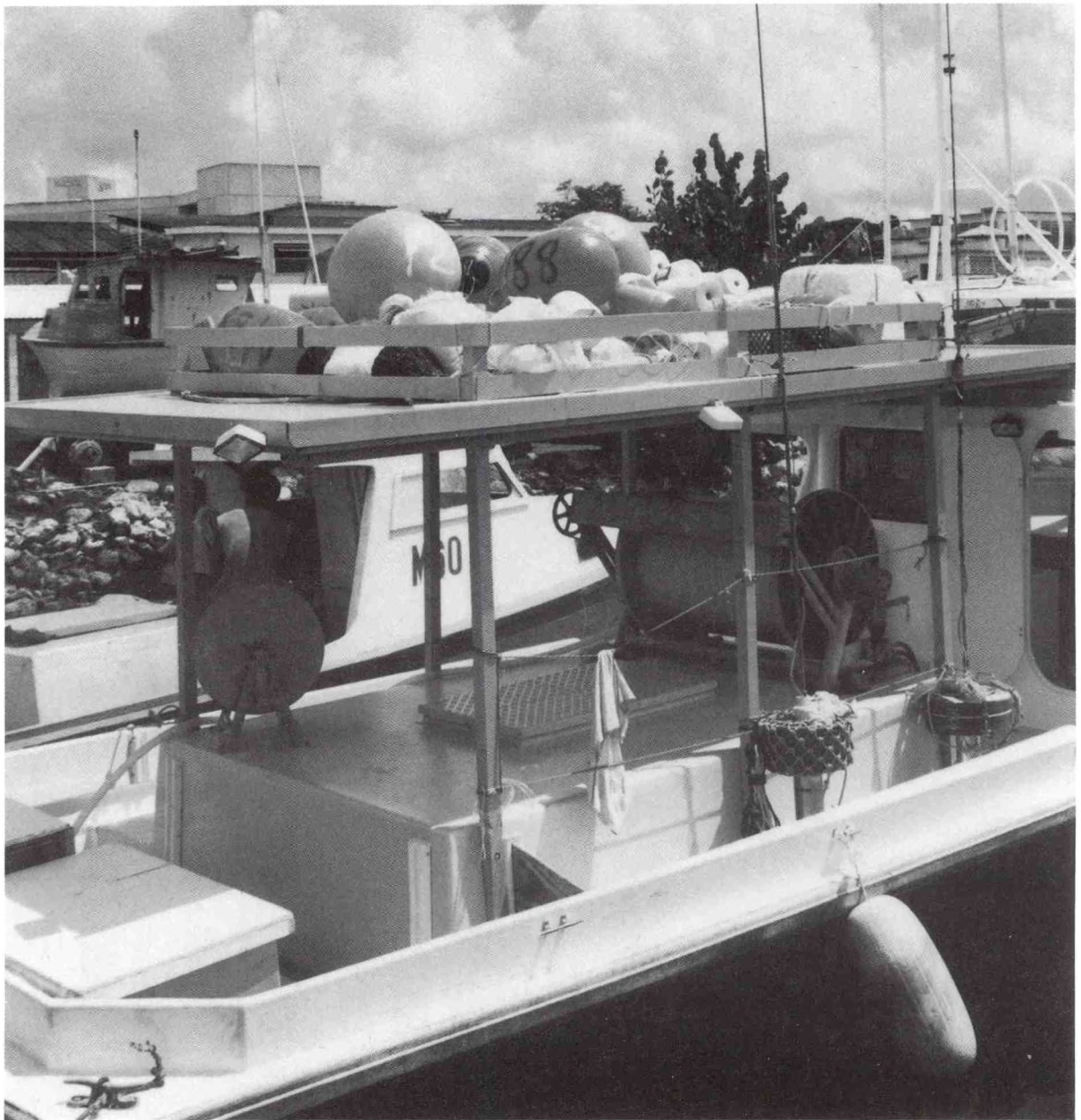
Photo 27.--This photo shows the typical arrangement of the aft deck on a Barbados longliner. Notice the reels, ice hold, hook boxes, upper deck gear pound, and radio buoy. Dennis Weidner
