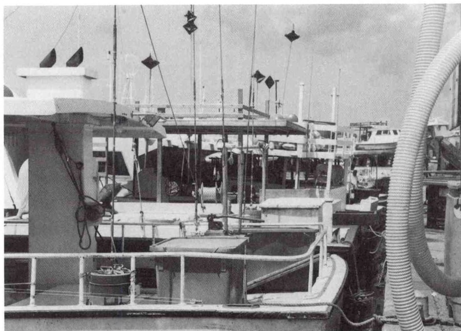
Photo 35.--The "Hi-Flyers" to help locate the line can be seen on these longliners. The tube at the right is for funnelling ice into the hold. Dennis Weidner
