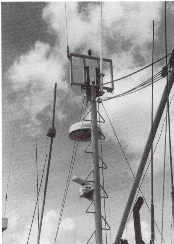
Photo 20.--This Barbados longliner is equipped with a short and long range radar as well as communication antennas. Dennis Weidner
