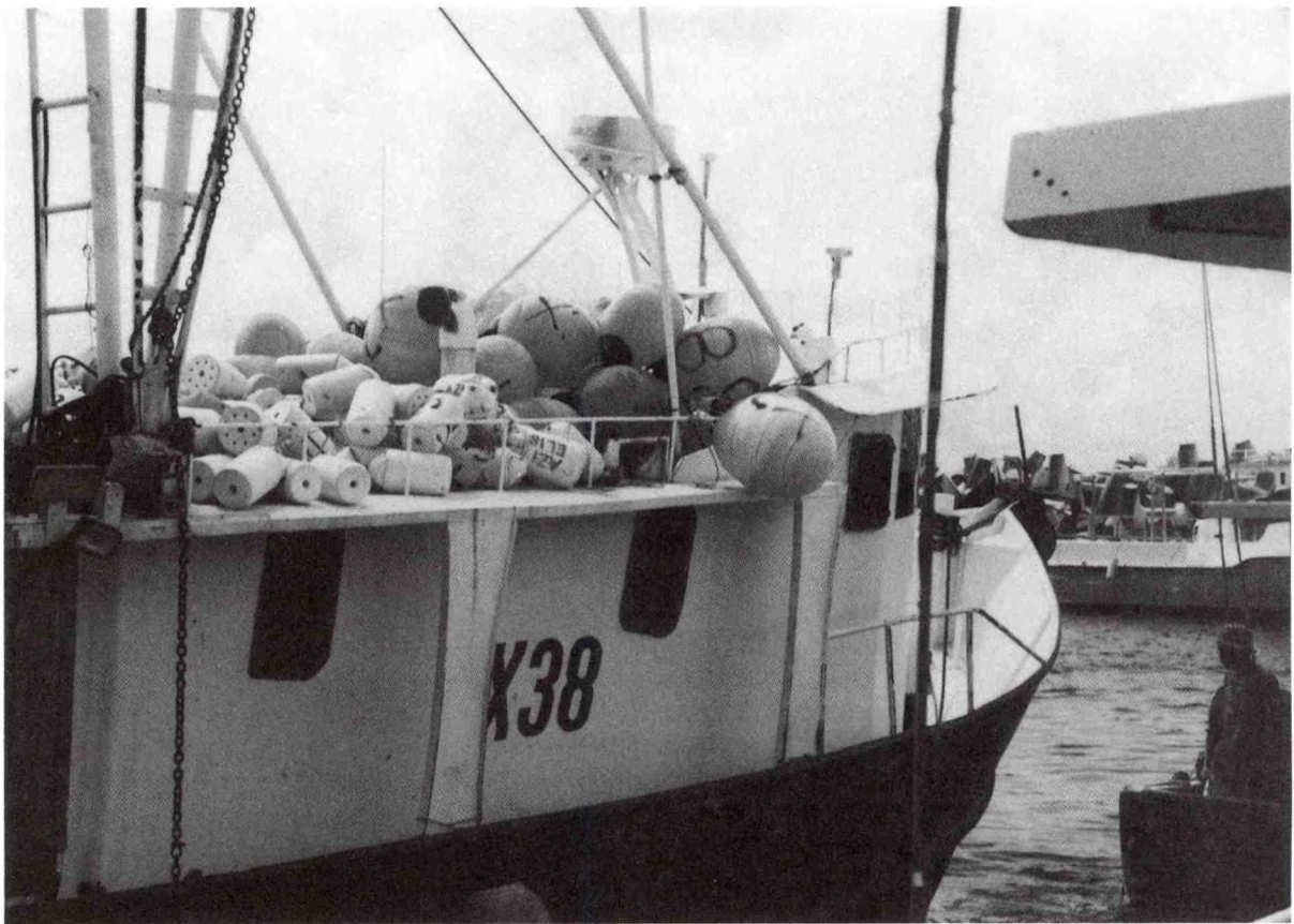
Photo 18.--The longline fishermen stow their gear on the upper deck so that the main deck is clear and uncluttered. Dennis Weidner
