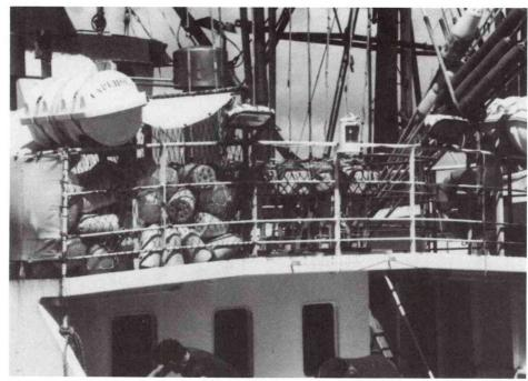
Photo 46.--Fishing gear stowed on a Portuguese longliner operating out of Natal. Note the floats, buoys, radio transmitters, and signal flags. Dennis Weidner Dennis Weidner
