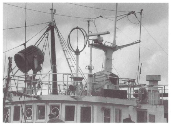
Photo 60.--Search lights are used at night while setting longlines. Also note antennas and radar equipment. Dennis Weidner
