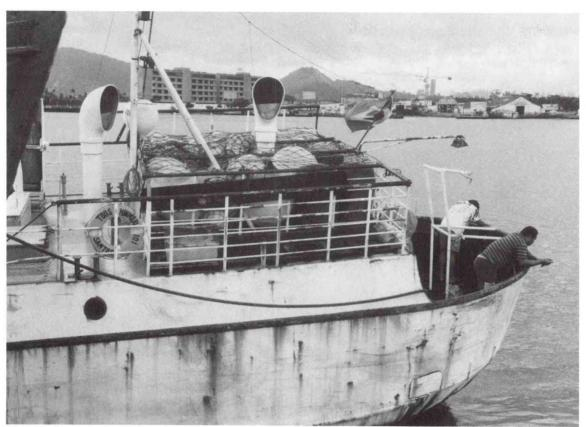
Photo 29.--Stern of a Brazilian longline with stowed float gear. Note open stern, making operations in inclement weather difficult. Dennis Weidner
