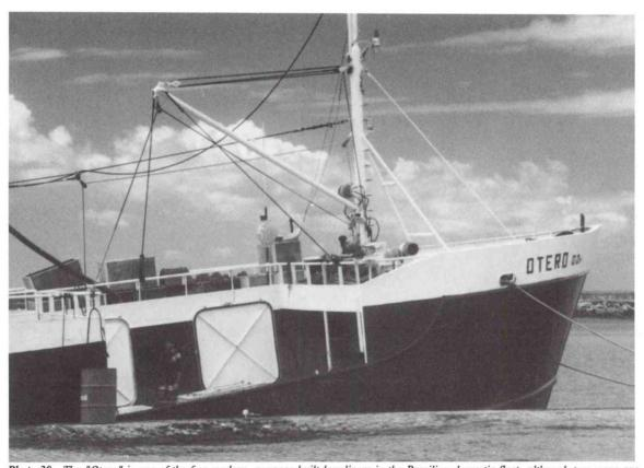
Photo 30.--The "Otero" is one of the few modern, purpose-built longliners in the Brazilian domestic fleet, although two more are under construction in 1988. Dennis Weidner
