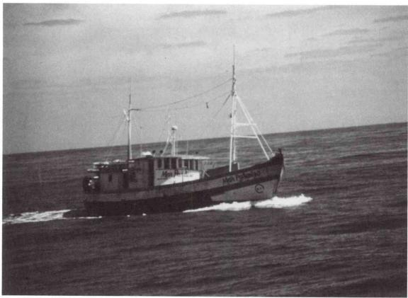
Photo 25.--Most Brazilian longliners are vessels converted from other fisheries. This is a former wooden trawler converted as a bottom longliner for operations off São Paulo State. Fabio Olmos
