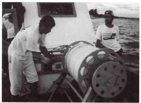
Photo 73.--Small longline drums like these are being installed on artisanal boats in Brazil. This one is being used by UFRPe for research on longline gear and methods. D. Weidner
