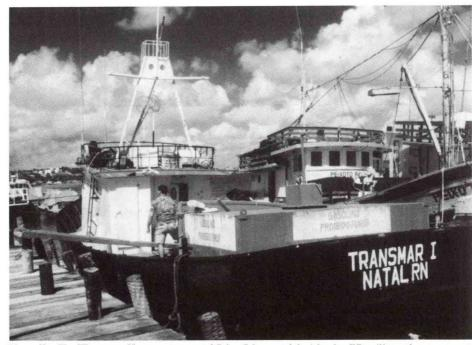
Photo 48.—The "Transmar I" targets tunas and flying fish around the islands off Brazil's northeastern coast, the long trips necessitate the added on-deck fuel tank. Dennis Weidner
