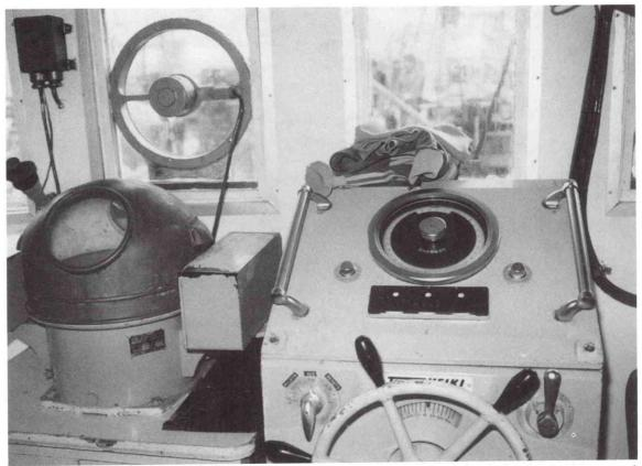
Photo 28.--Wheel house of the "Taimei Maru 3". Note the magnetic compress to the left and the wheel equipped with a gyroscopic compass and auto pilot. Dennis Weidner
