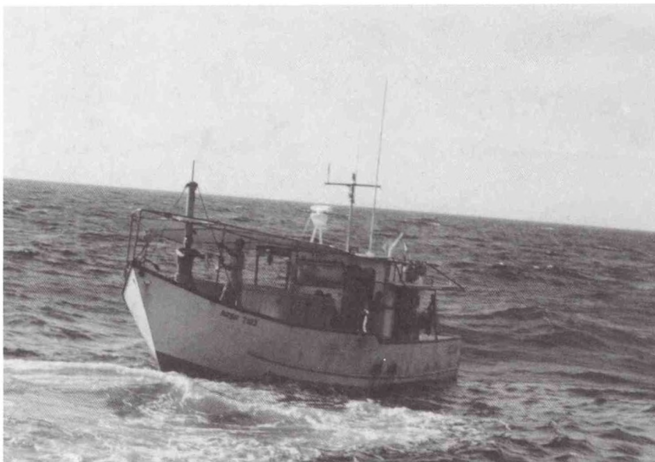
Photo 7.--An artisanal longliner targeting billfish in the water around Margarita Island. Note the on-deck hold. Freddy Arocha.
