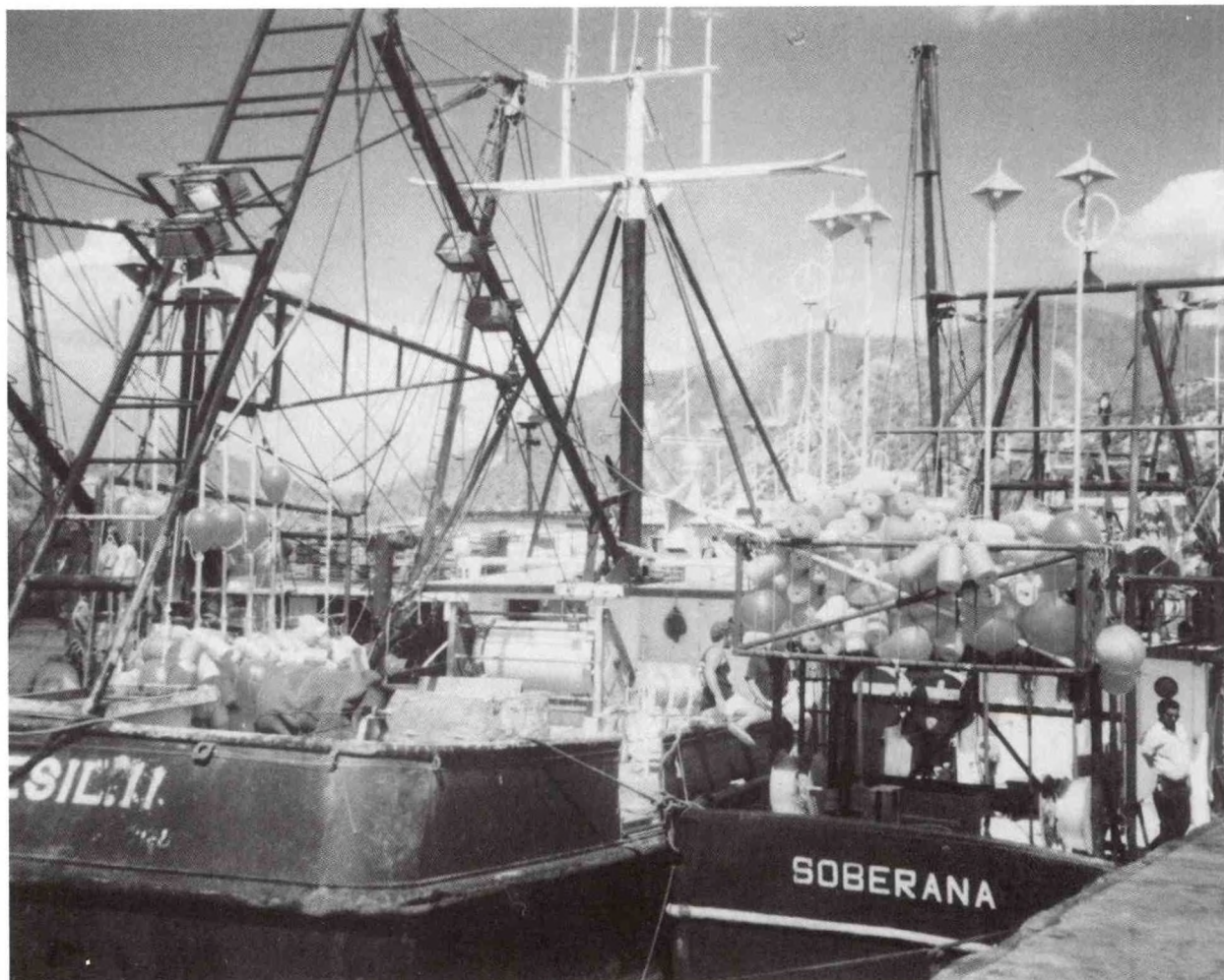
Photo 21.--These two longliners were active during the early 1990s. Note the floats and longline drums equipped with monofilament lines. Freddy Arocha.
