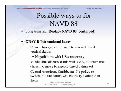
Although the idea of a GNSS/geoid vertical datum will mean realization errors generally no better than 2 cm at any given location, this is better than NAVD 88 which has leveling error build up away from Father point. Additionally, the ability to know the datum through a single GNSS receiver at any point of convenience will mean that leveling from existing bench marks to "bring in" the datum will no longer be necessary.
