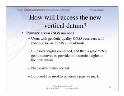
Multiple questions come up about using the new vertical datum. Two examples are given in the next few slides. The first is the example of how the new datum will address subsidence, say for floodplain mapping. The second example is about how the datum will be accessable when there aren't bench marks in the immediate region of interest. Both examples rely on this simple formula:
