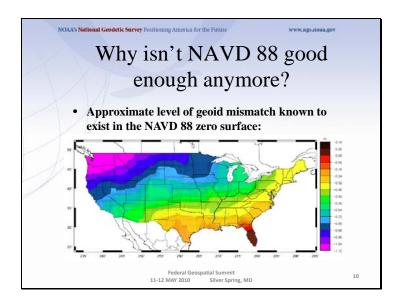
This map reflects the sort of height changes that users could expect if NAVD 88 were replaced with a geoid-based vertical datum. This is only a large scale approximation and should not be used as an absolute guide.
