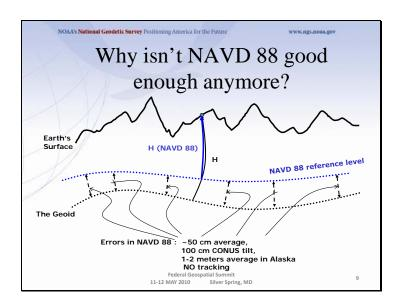
This slide shows what NGS now knows about the error in NAVD 88 itself. Using a continental geoid computed from the GRACE satellite, a bias and tilt in NAVD 88 has been computed using GPS derived ellipsoid heights on NAVD 88 bench marks. These are now known errors that exist in all NAVD 88 bench marks. This datum realization error, relative to the geoid, is over and above the errors from marks moving.
