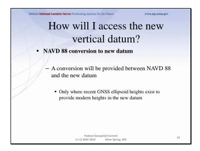
In areas where a brand new (relatively speaking) GNSS based ellipsoid height has been determined at an NAVD 88 bench mark, that data will allow for NGS to convert to the new datum. The more of these points that can be determined right near the time of the new datum's release, the better will be the conversion.
