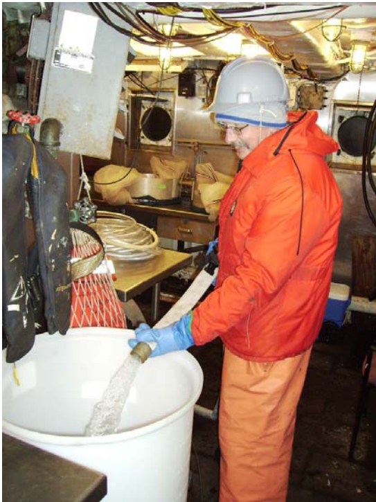
Figure 4. Microbial Sample Barrel being filled by De-watering Pump aboard Delaware II 0602 Cruise.
