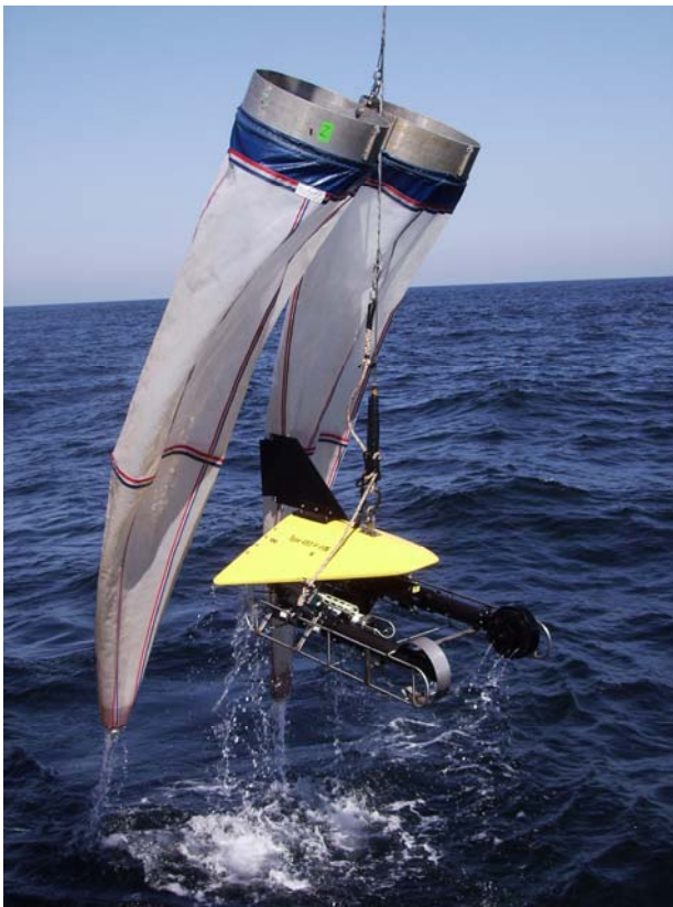
Figure 2. 20 cm Bongo Sampler mounted above a 61 cm Bongo Sampler.
